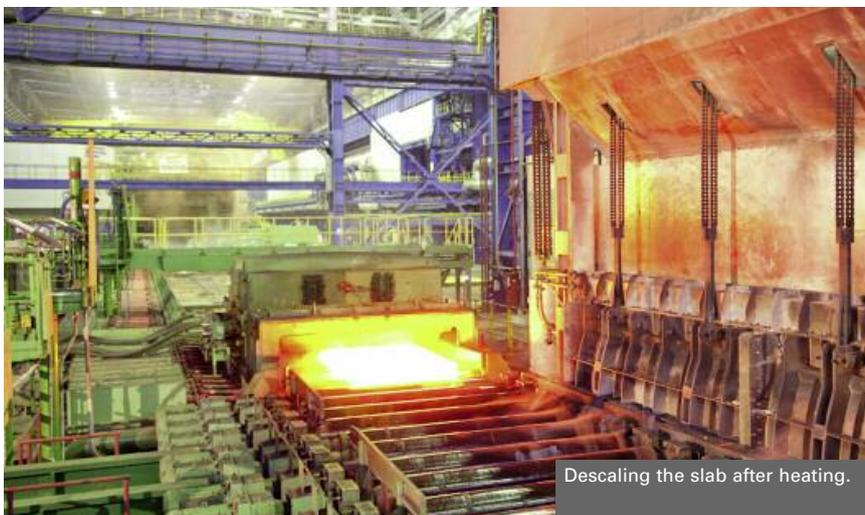
Descaling the slab after heating.
