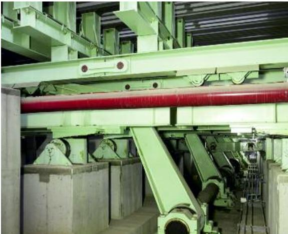
The walking beam mechanism transports the plates without damage.
