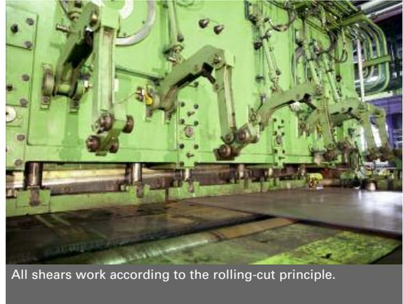
All shears work according to the rolling-cut principle.
