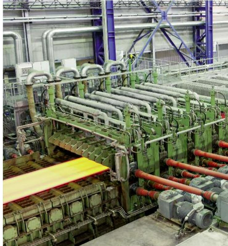
The combined spray and laminar cooling, a highly flexible metallurgical tool.
