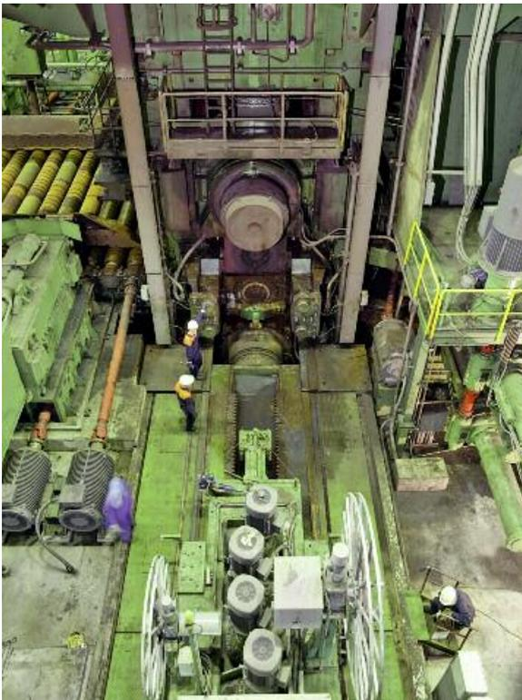
Work-roll changing is fully automated with a locomotive.
