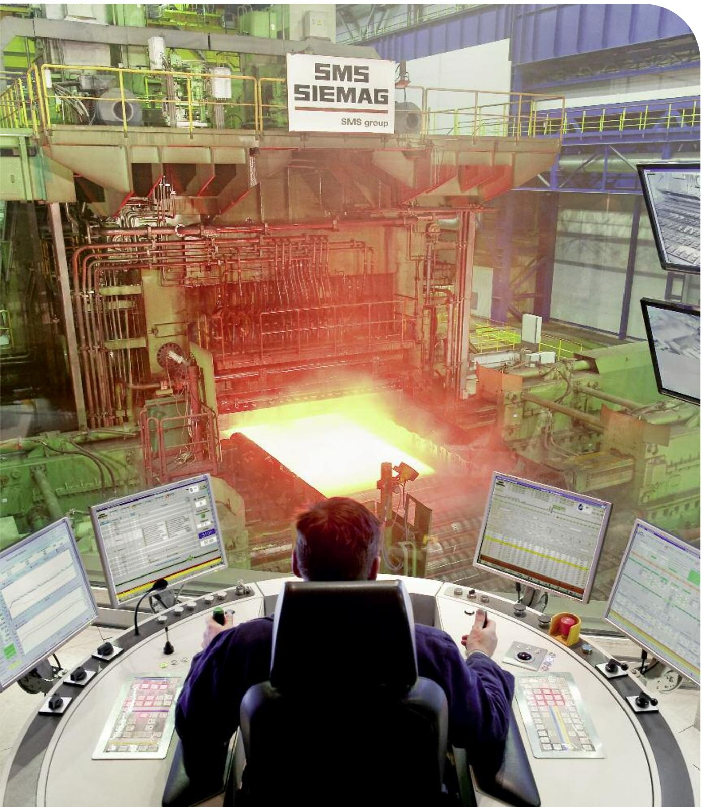
The ergonomically designed control desk enables an unrestricted view of the rolling process.
