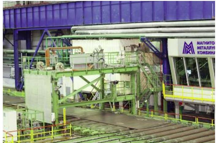
Ultrasonic scanner and plate measuring system downstream of the cooling bed.
