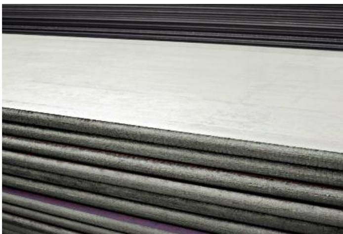
Plates between 50 and 160 mm thickness roll off the line before the cooling bed.
