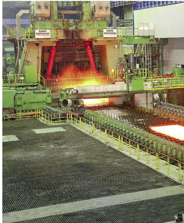
Multi-plate rolling with up to six plates was standard after just a few months.
