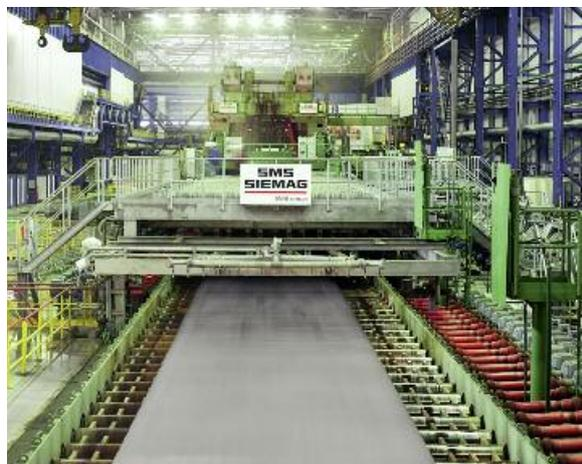
The cooling system and mill stand must form a unit for thermo-mechanical rolling.
