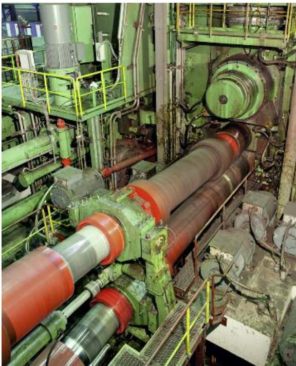
The flat-neck spindles feature length compensation for shifting the work rolls with the CVC® system.
