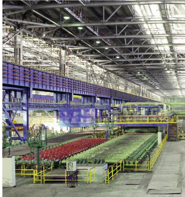
The thermal treatment line with the hardening furnace and quencher (left) and the normalizing furnace (right).
