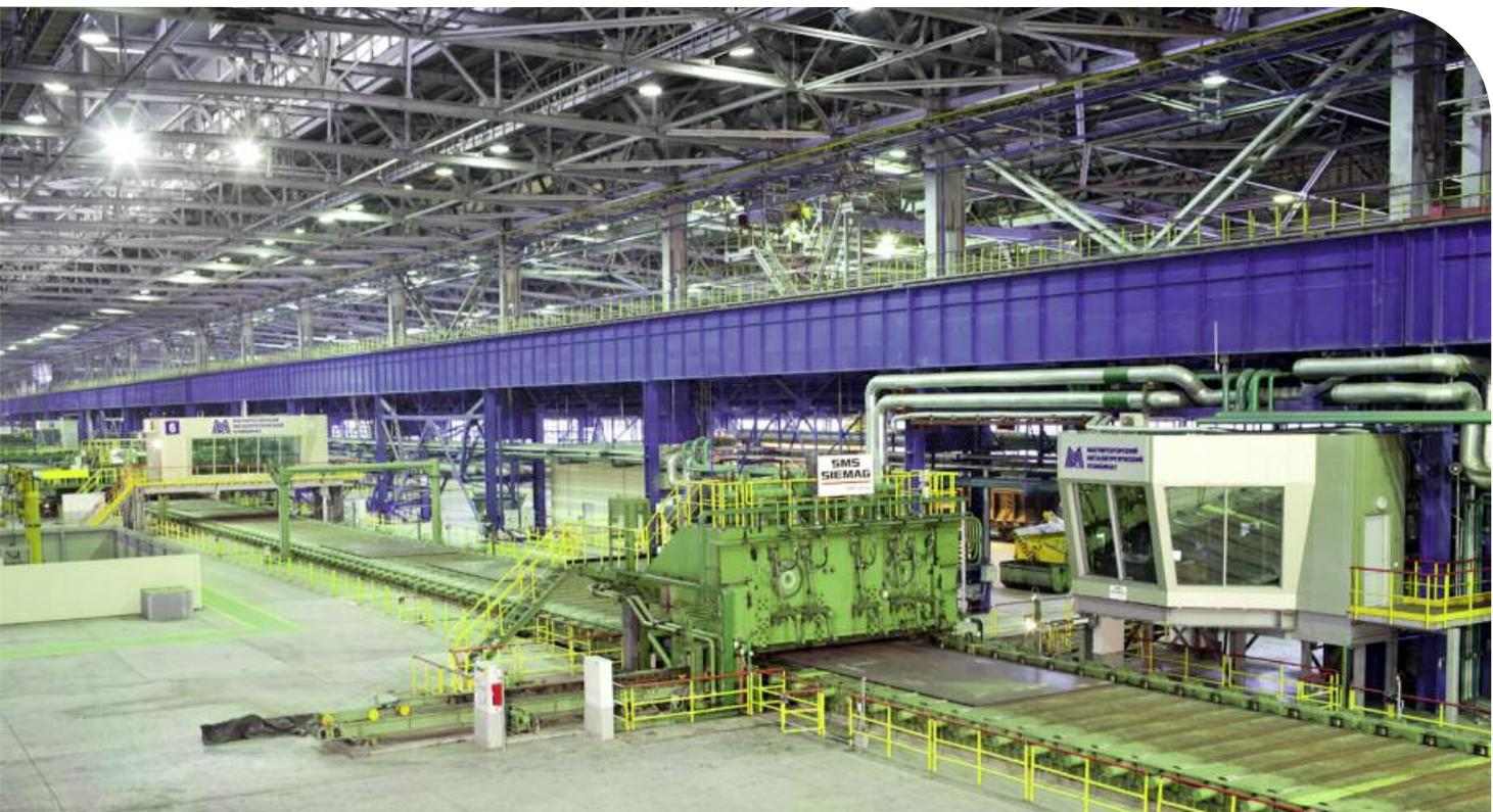
Cropping shear as well as slitting and trimming shear (in the background).
