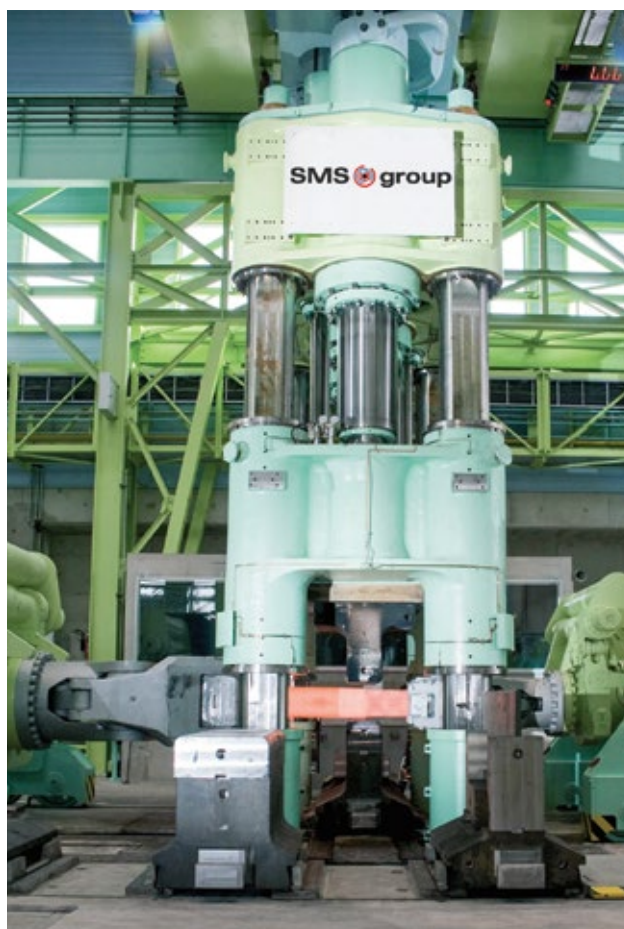
An open-die forging press of the same design as the one being supplied to Daye Steel.
