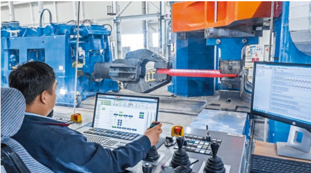
The new 63/80-MN high-speed open-die forging press in operation at WST.
