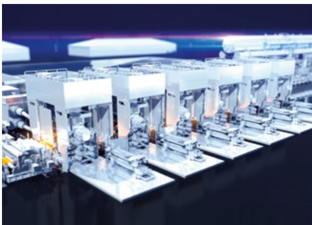
The CSP® finishing mill will consist of six rolling stands designed for thermo-mechanical rolling and the rolling of API grades X80.
