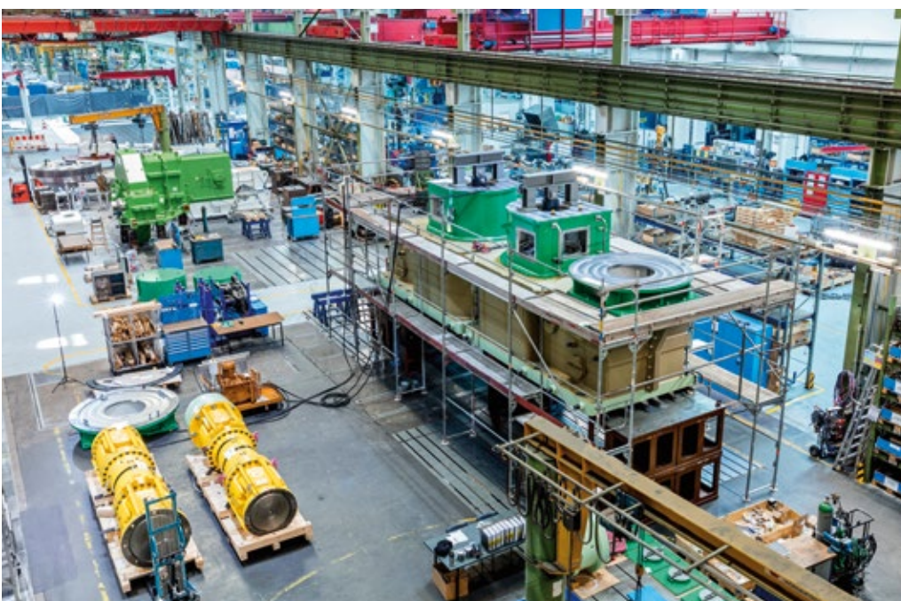
Pre-assembly of the complete edger gear-box and preparation for acceptance by the customer.
