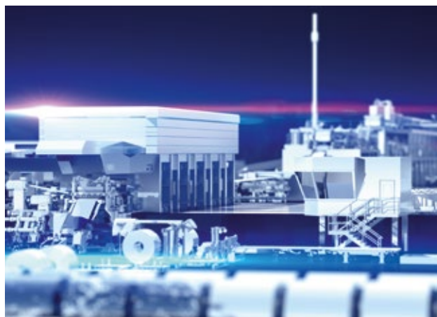
The continuous pickling line/tandem cold rolling mill downstream of the CSP® plant will have five stands and apply the latest turbulence technology.
