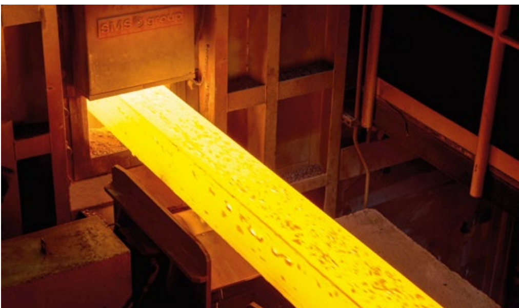
Billet being discharged from the new reheating furnace at Nucor Marion.
