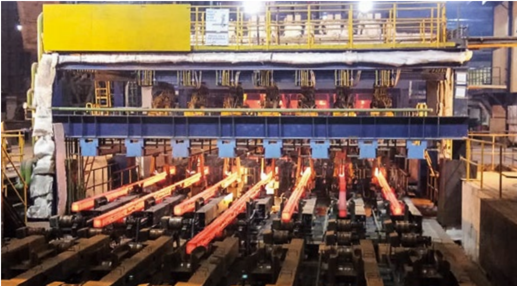
The new high-speed, seven-strand combi-caster in operation at JSPL Angul in India.
