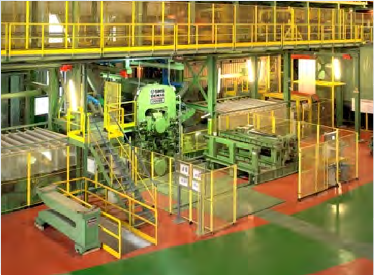
Inline and Offline Skin Pass Mill for CAPL, complete with strip and roll polishers, including dust suction systems.
