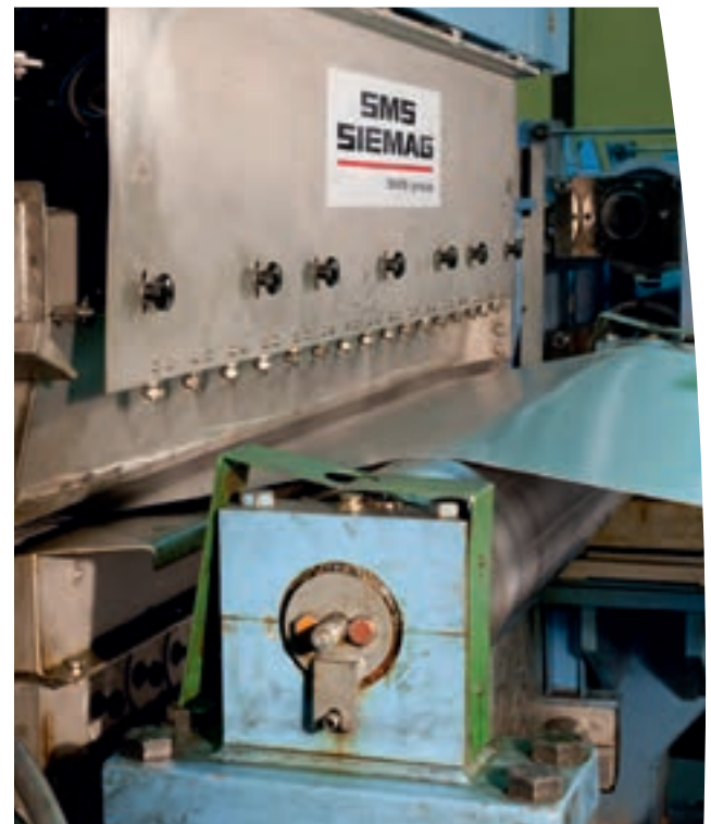
Atomizing the lubricant by compressed air.
