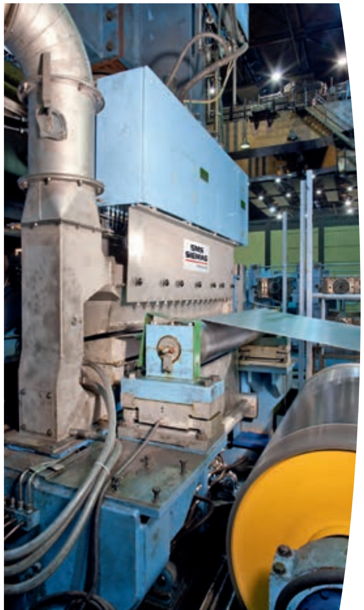
Entry: Atomizing of the lubricant by compressed air. X-shape flatness measurement roll.
