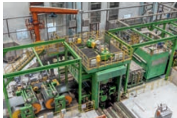
ISPM in CGL: S-roll sets support the strip tension necessary for the skin-pass process.
