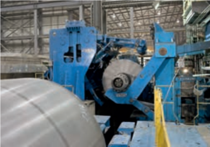
Strip preparation, uncoiler and tension roll set of a running, comparable offline skin-pass mill
