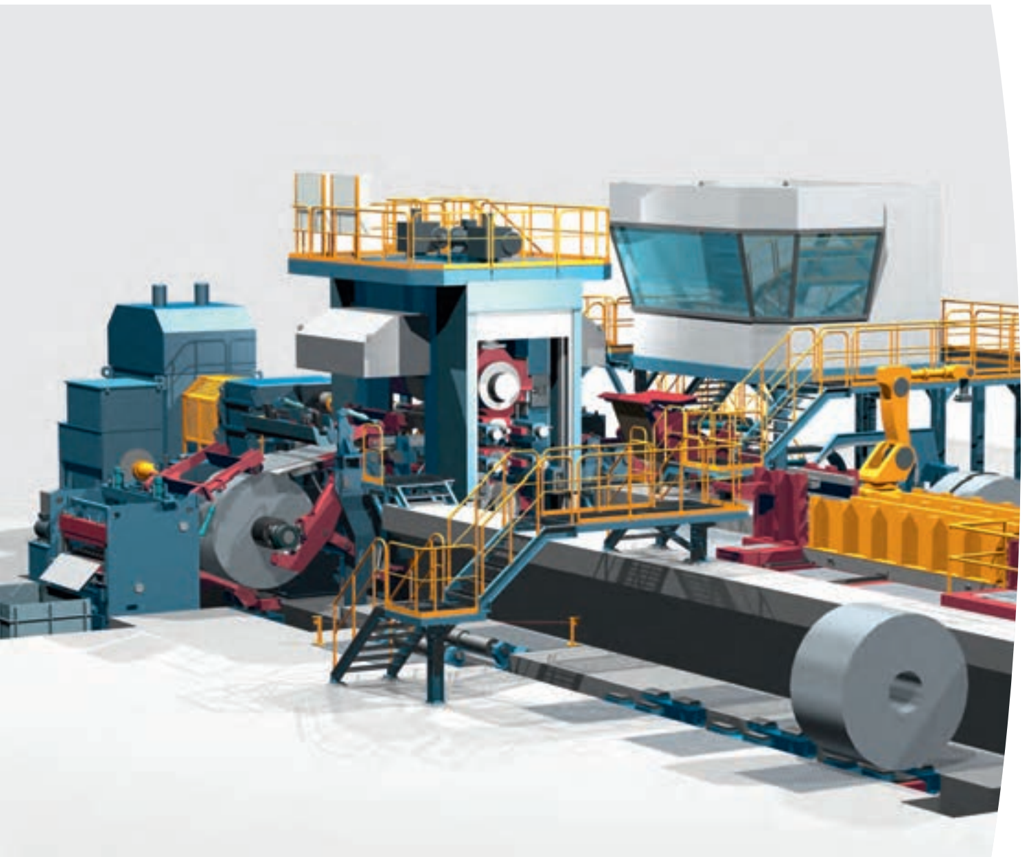
Concept of a similarly configured offline skin-pass mill from SMS group.
