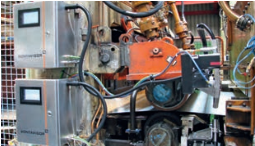
Online measurement system for measuring the residual oil content.
