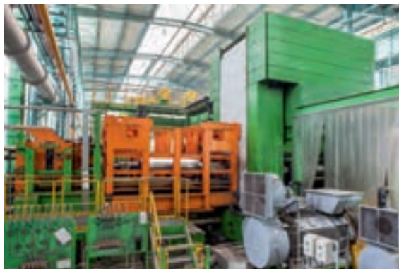
Drive side. The roll shift takes place in push-through operation.
