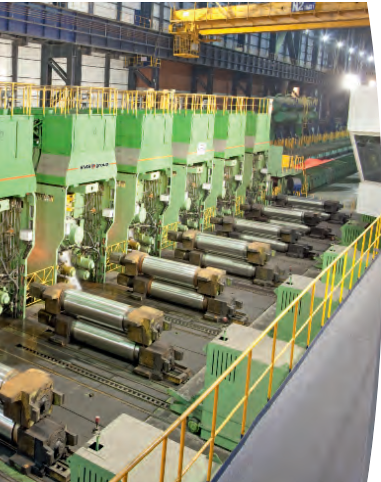
Automatic work roll changing in the seven-stand finishing mill.
