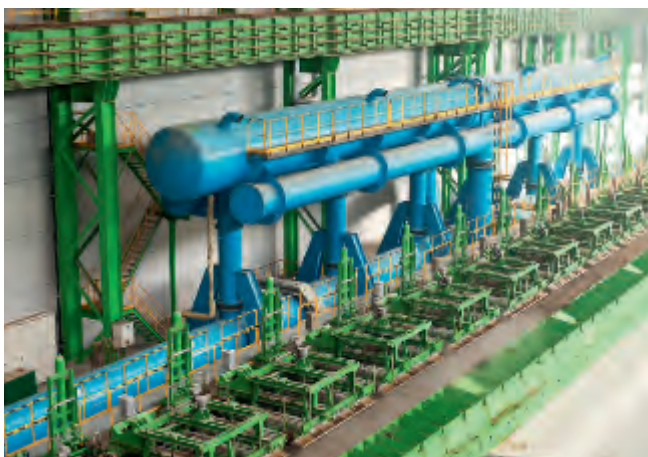
Laminar cooling system with edge masking.
