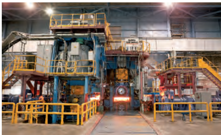
Two-high roughing stand with edger.
