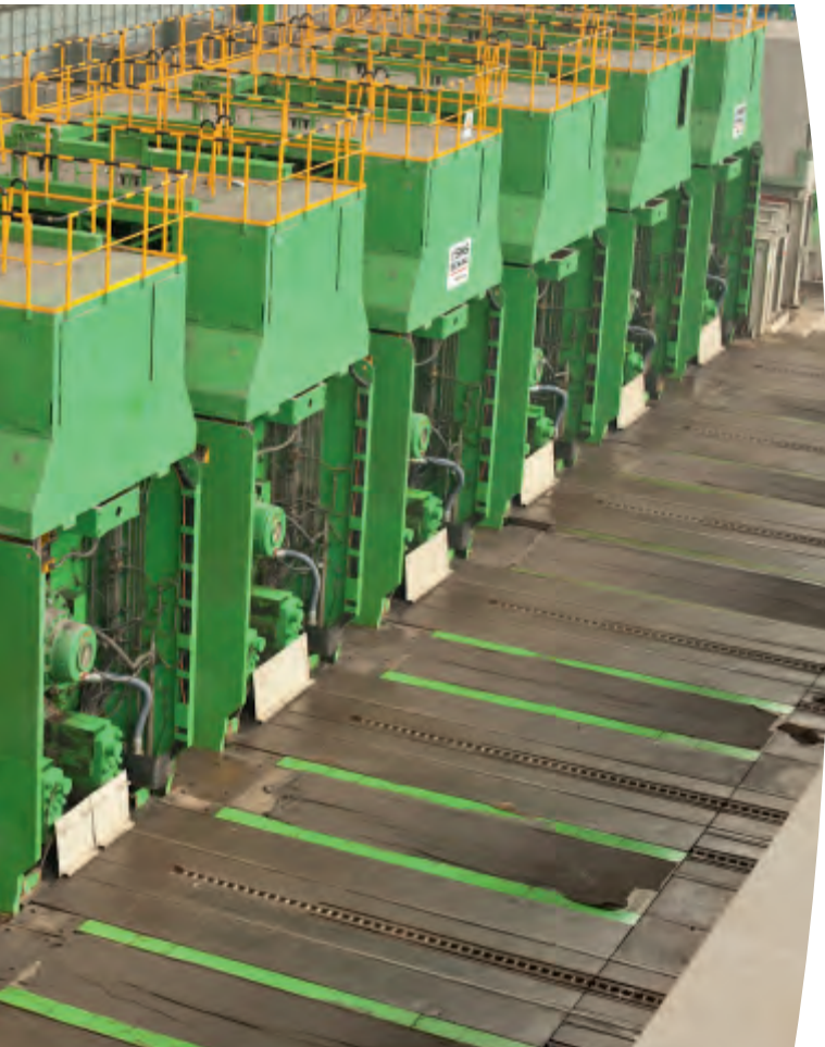
The hydraulic control systems are accommodated in protective housings in the utility platforms on the millstands.
