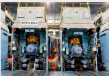
Finishing stands with CVC® plus technology
