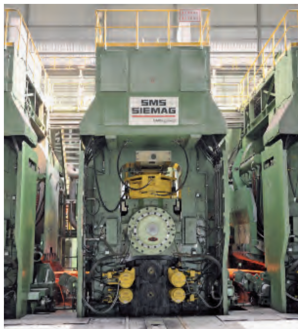
Left: Finishing stand with CVC®plus, work roll bending, and hydraulic roll-gap adjustment systems.
