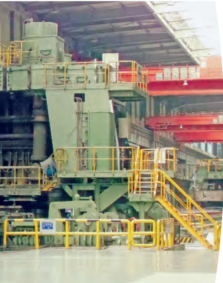
Roughing mill stand and edger.
