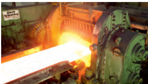
Drum-type crop shear.
