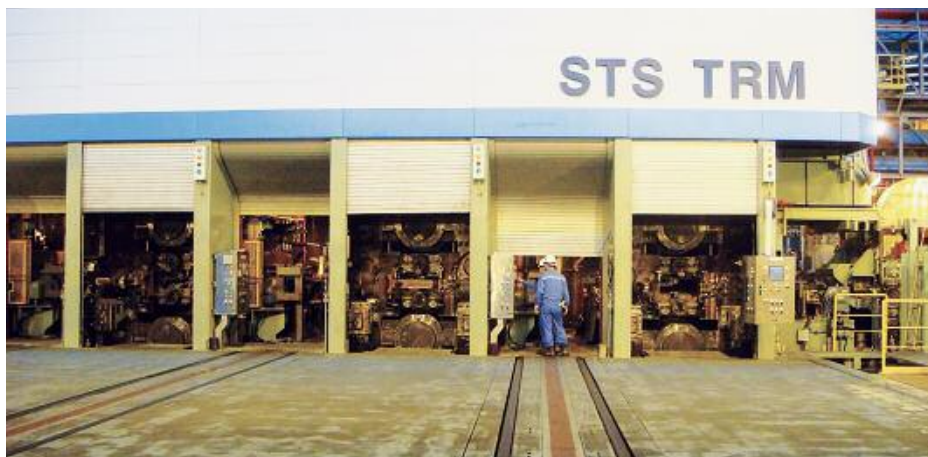
Continuous tandem cold mill with four 18-roll mill stands.
