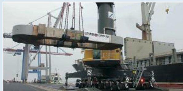
Delivery of a mill stand of the tandem cold mill to its final destination Osceola in the US federal state Arkansas.
