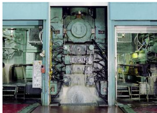
Housing window of six-high stand.
