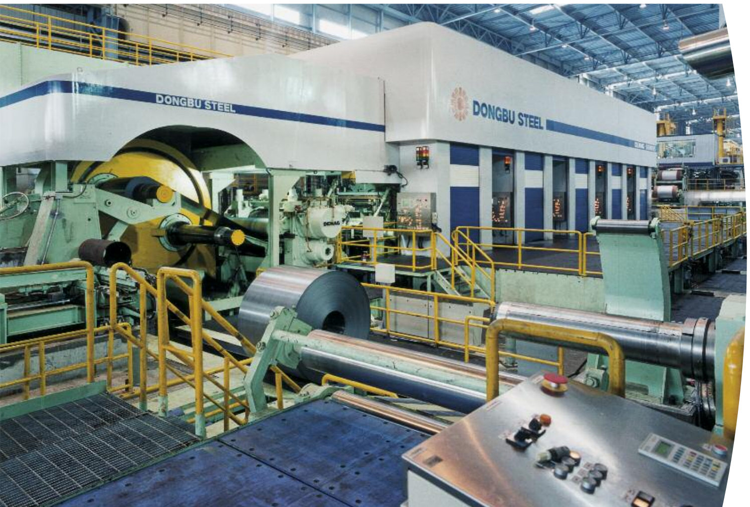
Exit end with carrousel-type reel.
