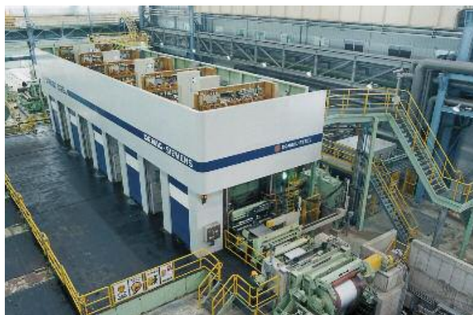
Entry end with coupling to the pickling line.
