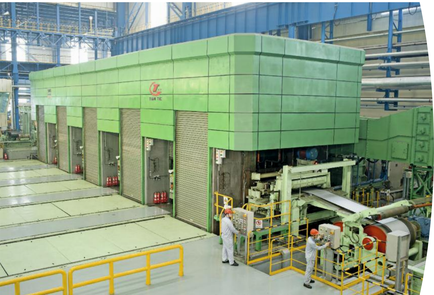
Entry end of the tandem cold rolling mill.
