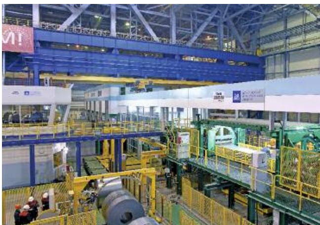
Tandem cold mill with inline inspection line („Rotary Inspect“).
