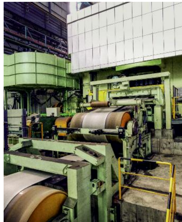
Entry section tandem cold mill.
