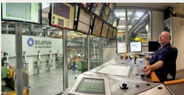
Integrated in the level 2 automation, for the first time TRC® was installed for the first time in the course of the modernization of a tandem cold mill
