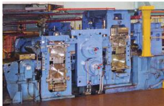
Drum shear with pinch roll units in the exit section.
