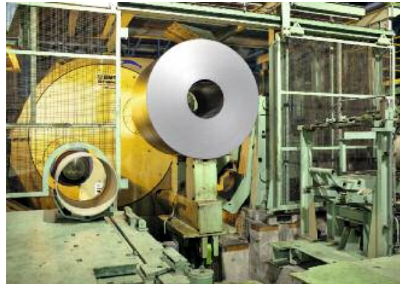
Removal of a coil from the carousel reel.
