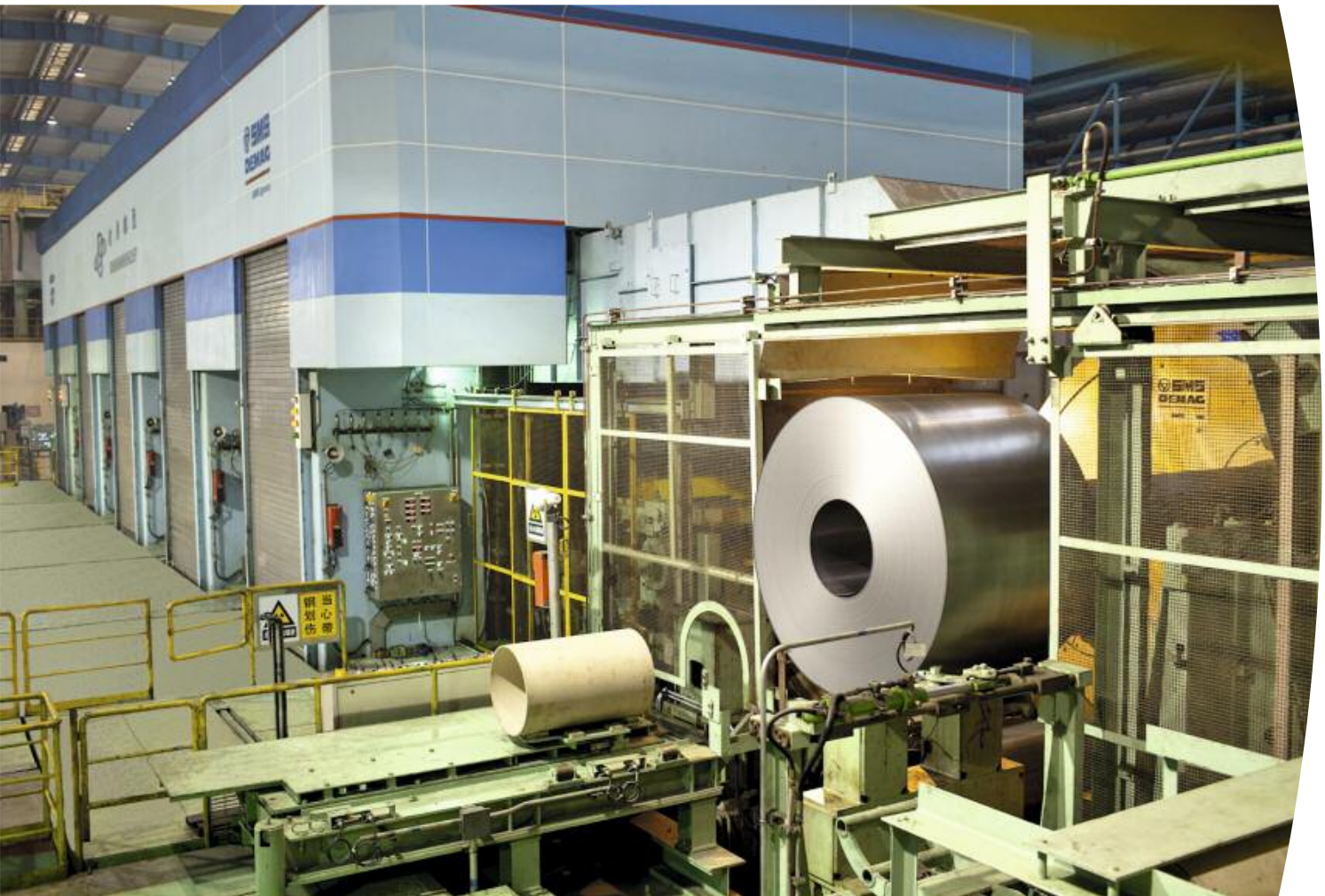
The tandem rolling mill with carousel reel.
