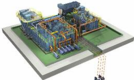
ECU-concept for a pickling line tandem cold mill with separate emulsion plants for rolling stands 1-4 and 5.
