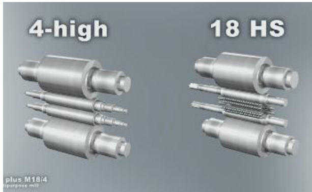
Changeable roll sets of the multipurpose mill.
