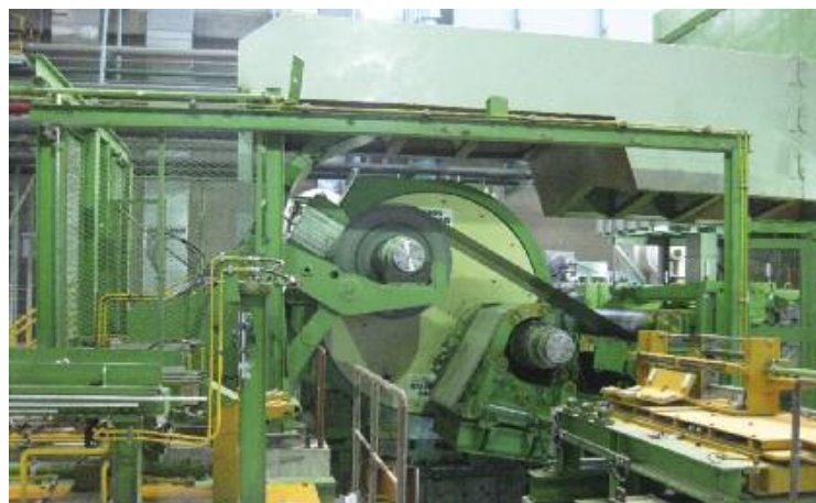
Continuous exit with carousel reel.
