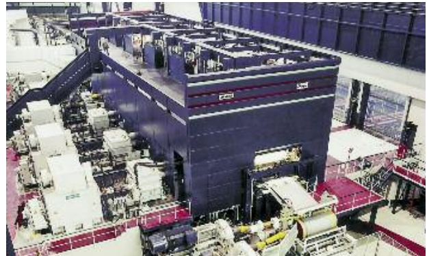
Clear arrangement of the hydraulic equipment in the mill stand top section.
