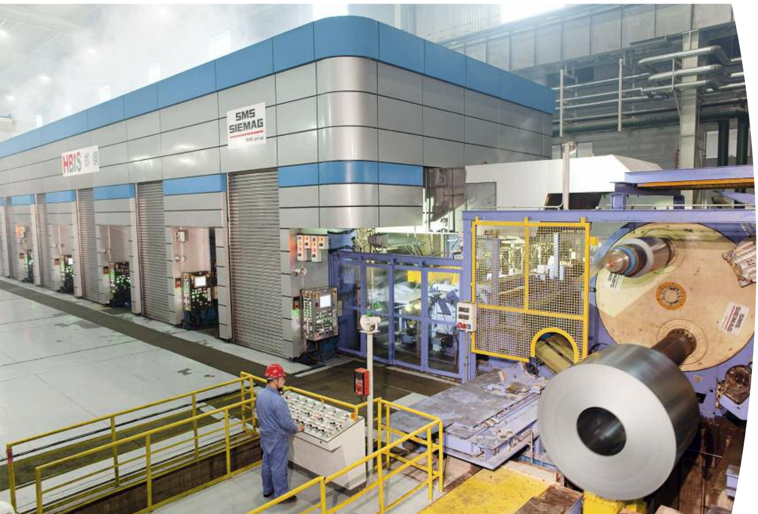
Coil evacuation from carousel reel.
