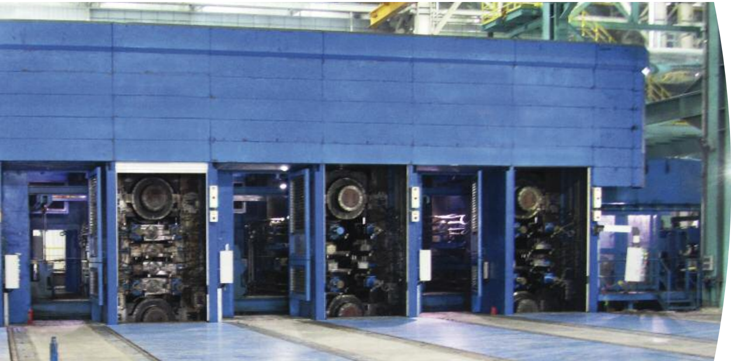
The tandem cold mill „TCM 400“ in the final stage of assembly.
