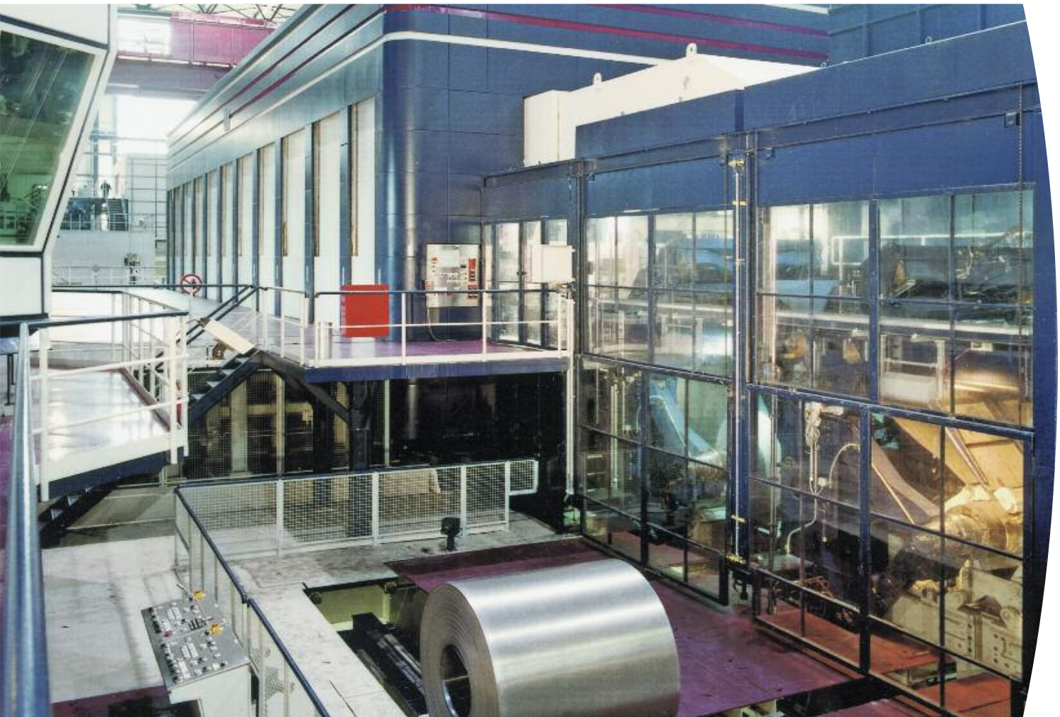
Exit side with two coilers and inline strip inspection.
