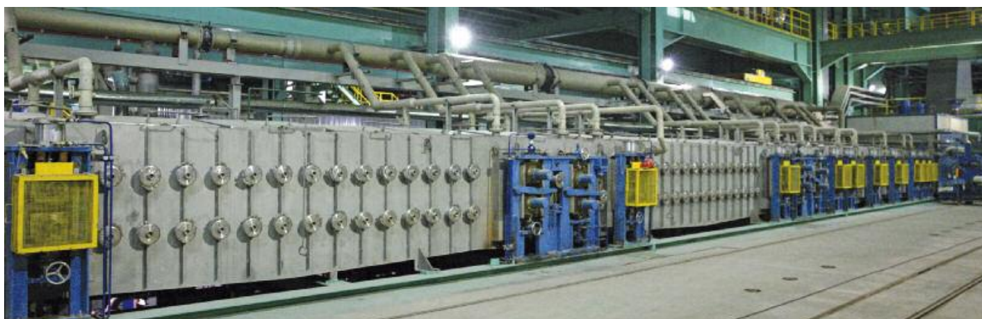
The downstream strip cleaning section removes emulsion residues from the surface of the finished stainless steel strip. It is characterized by compact design, efficient cleaning and low operating costs.
