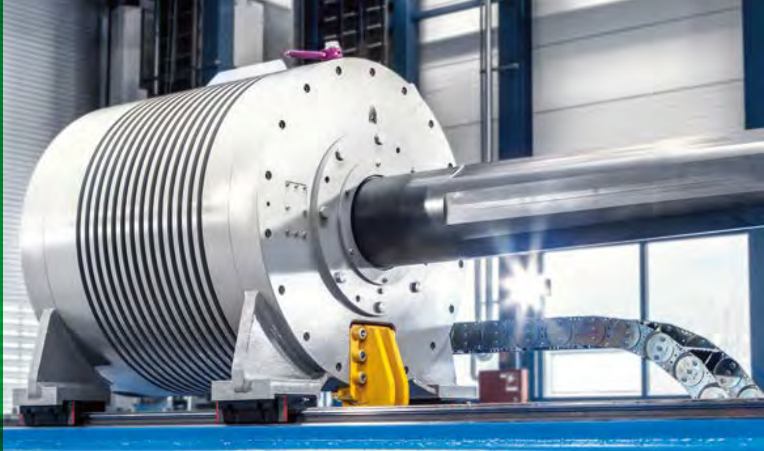
Compact edge-scrap coiler.
