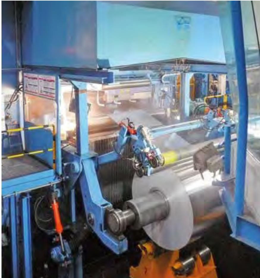
A double ironing roll supports the precise coiling of aluminium strip.
