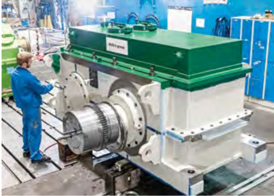
Final step in the manufacturing process: painting the new gear unit for Novelis Nachterstedt.
