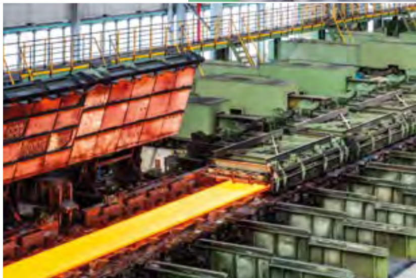
Heat insulation hoods reduce heat losses of the transfer bar.
