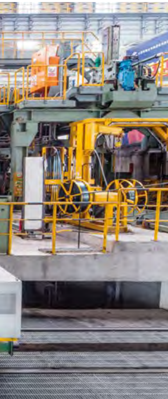
The high-performance hot strip mill is equipped with three downcoilers.
