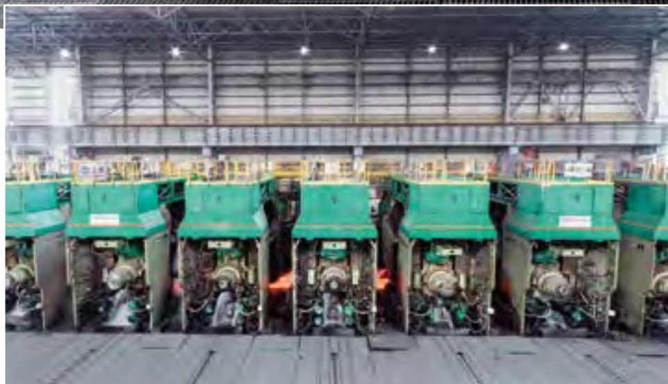
The seven-stand finishing mill rolls the transfer bar down to final thickness. All mill stands feature CVC®plus.
