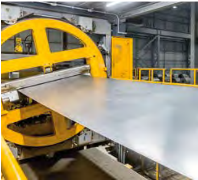
The new exit-side concept includes the cutting-edge Rotary Inspect offline inspection station permitting the fast and especially ergonomic inspection of strip top and bottom sides.
