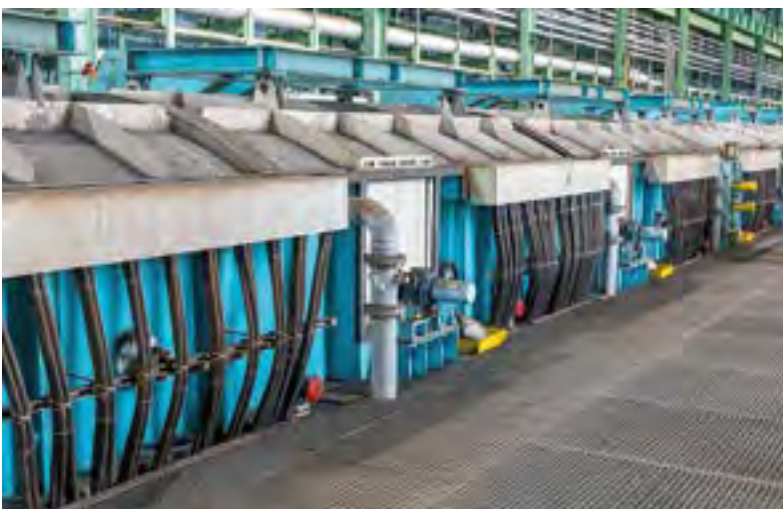
The pickling section will allow for a good pickling result at low consumptions and high speeds and include electrolytic sections, a turbulence pickling section as well as a rinsing area with oscillating brushes.
