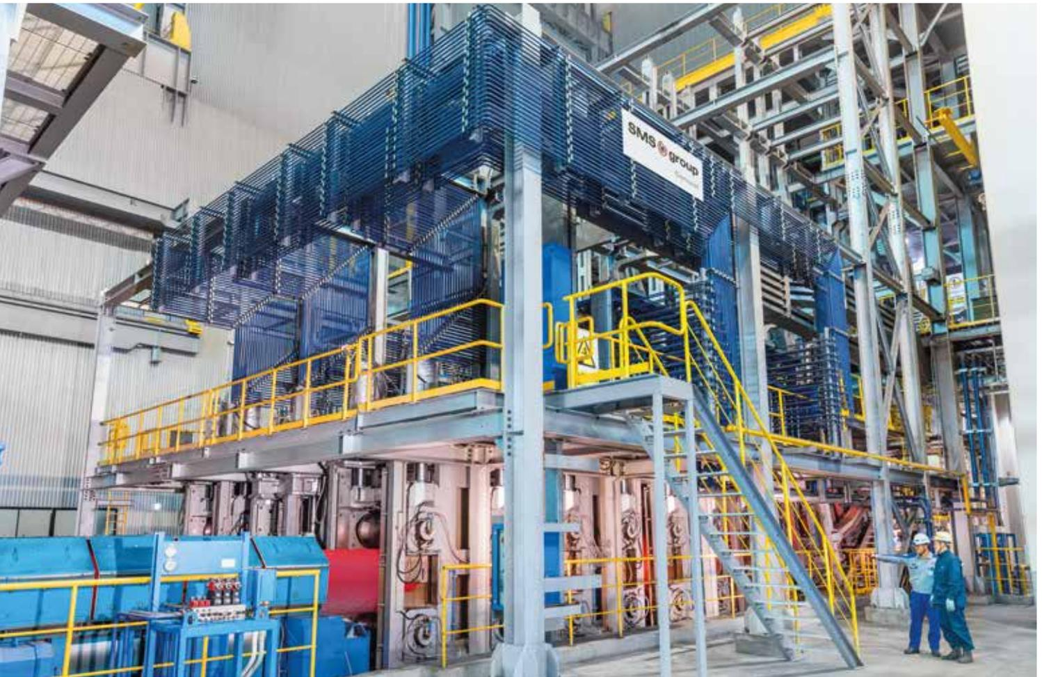
TAEWOONG in South Korea successfully casts round blooms of 1,000 millimeters in diameter on an SMS Concast machine.
