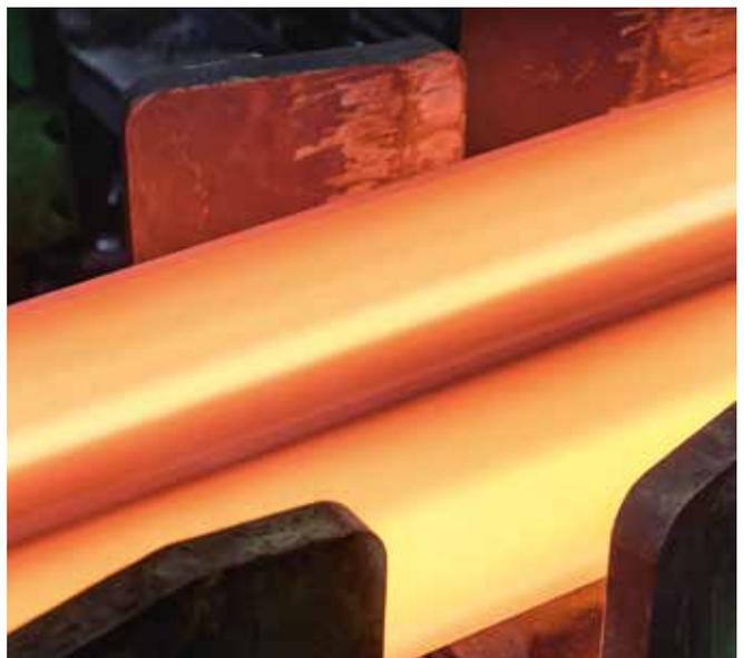
quenched and self-tempered is covered. Each cooling zone has its own pressure control system, so that the cooling rate for the whole area of the beam can be precisely adjusted for a homogenous temperature distribution over the beam. The QST process is suitable for beams with a minimum thickness of 25 millimeters. ♦
