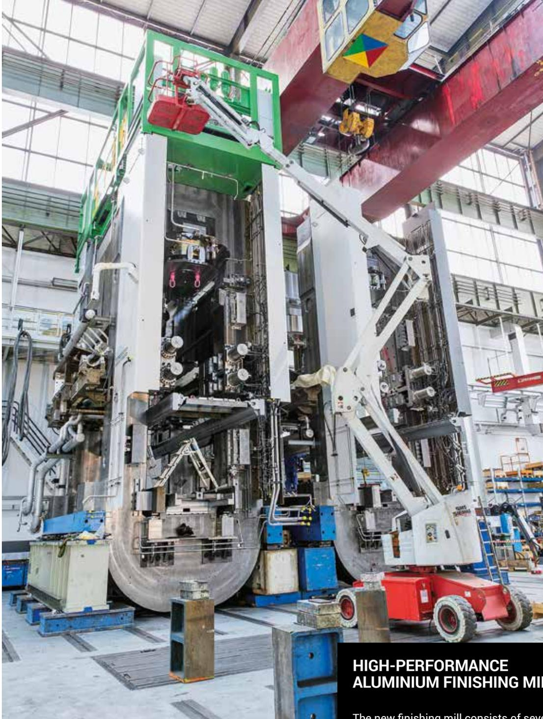
Preassembly of the aluminium-hot rolling stands. Pre-assemblies of several hundred tons total weight are possible in the workshop in Hilchenbach.
