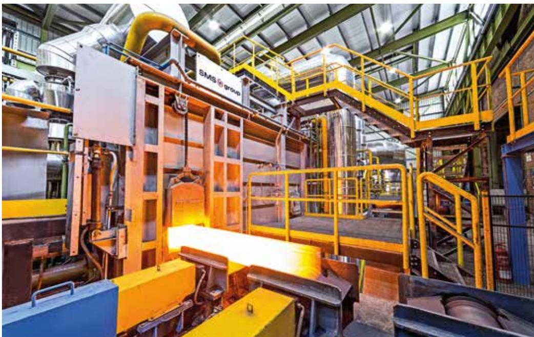
SMS group will increase the capacity of the walking beam furnace at Sidenor Basauri from 85 to 130 tons per hour.
