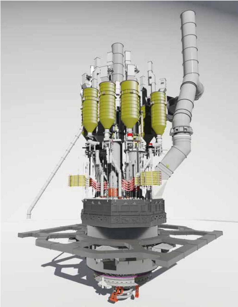
Latest development in rotating DC furnace technology for Si-metal.
