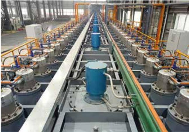
Radiant tubes heat the furnace to maximum 850 degrees Celsius.
