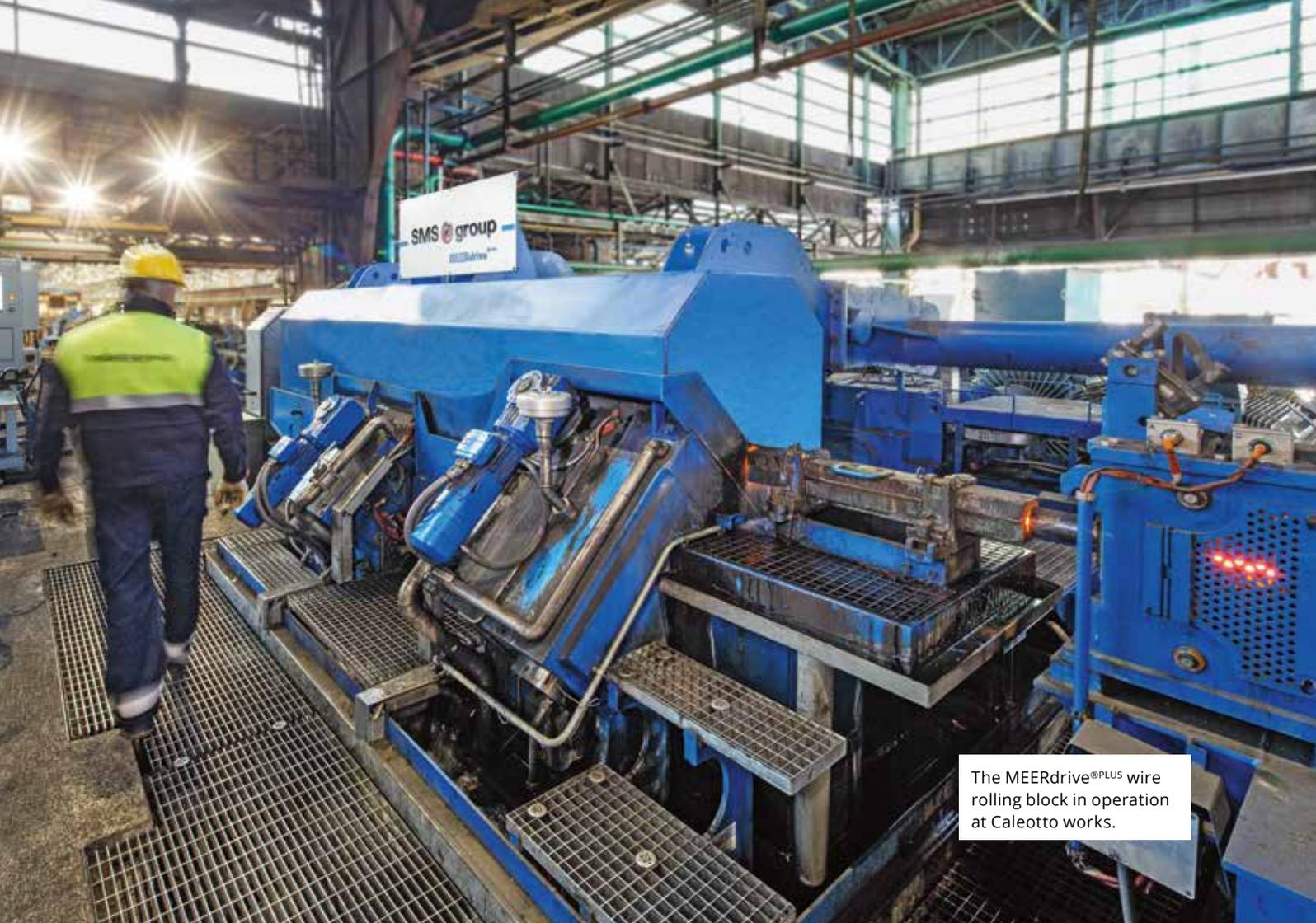
The MEERdrive<sup>®</sup>PLUS wire rolling block in operation at Caleotto works.
