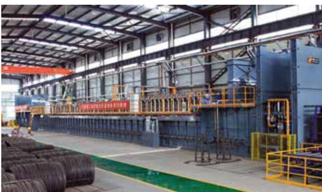
The furnace has a total length of 80 meters.
