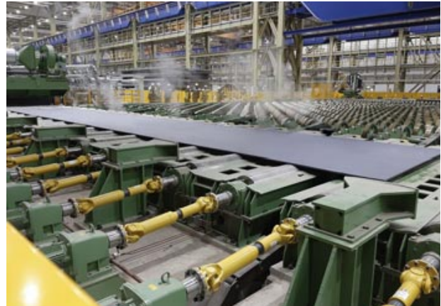
Exit-side view of the X-Roll® MultiFlex-Quench as the core component of the plate heat treatment line from SMS group.
