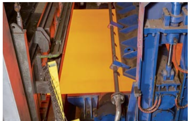
Excellent temperature uniformity of the heated plate at the point of transition to the quench
