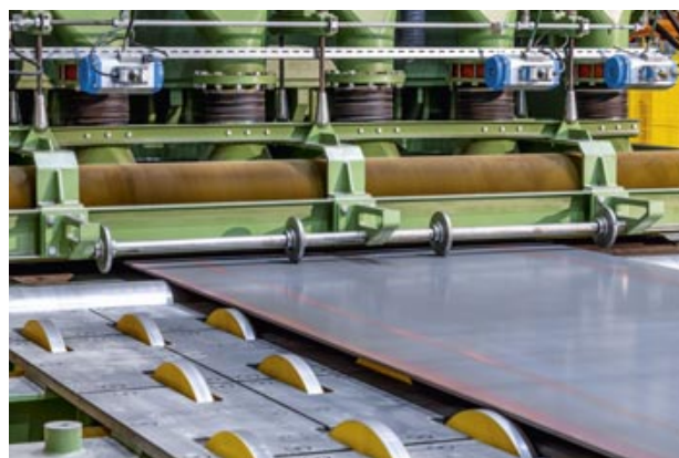
X-Roll MultiFlex-Leveler exit side with flatness measuring table.
