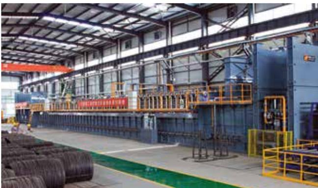
The furnace has a total length of 80 meters.
