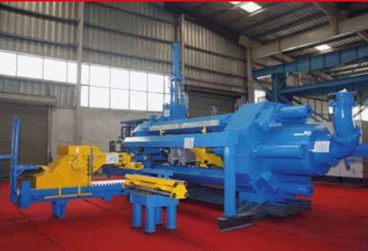
An 18 MN extrusion press „Made in India“, ready for delivery to the customer.
