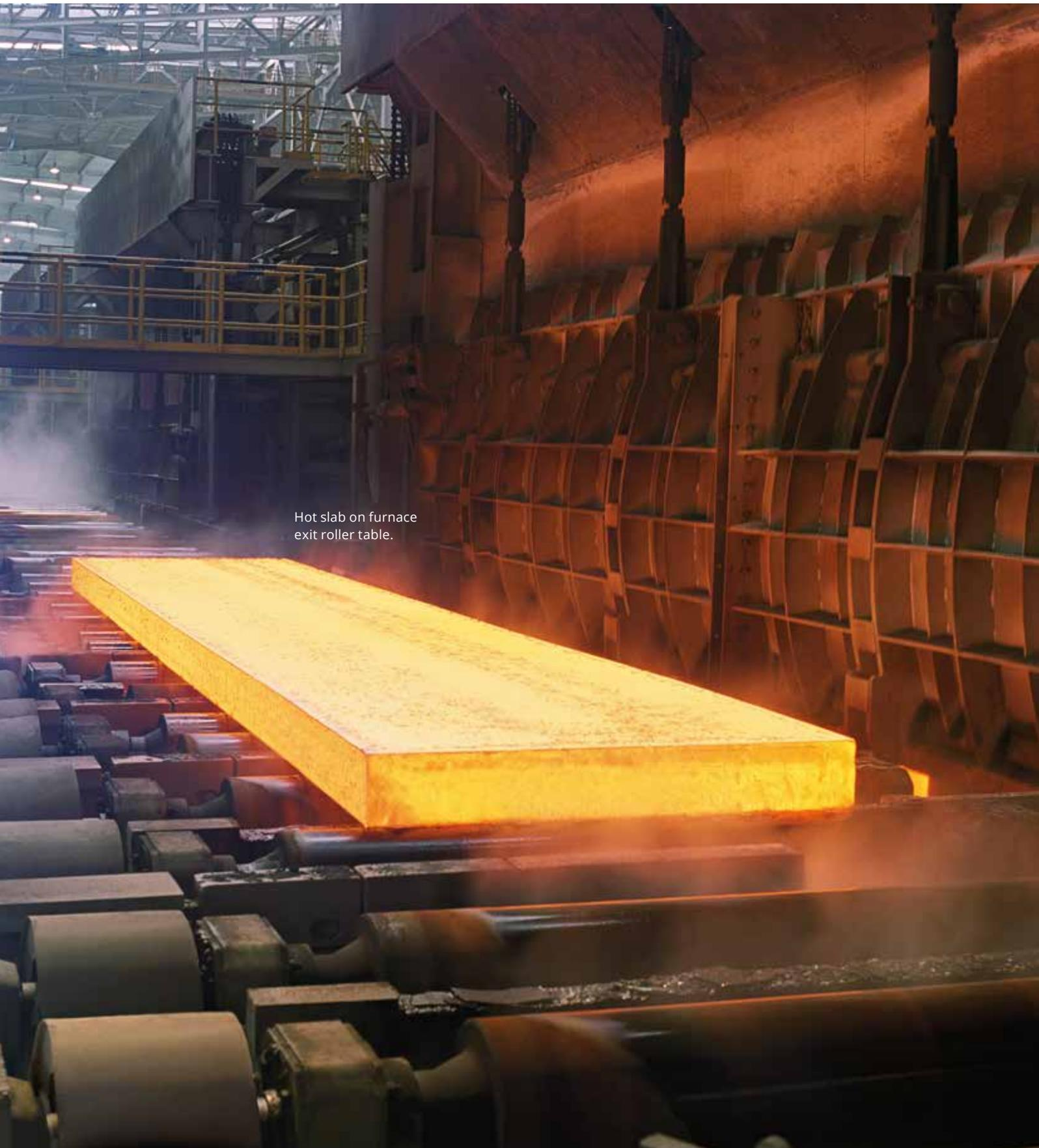
Hot slab on furnace exit roller table.
