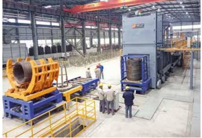
In the entry section, the coil stacks are continuously fed to the furnace.
