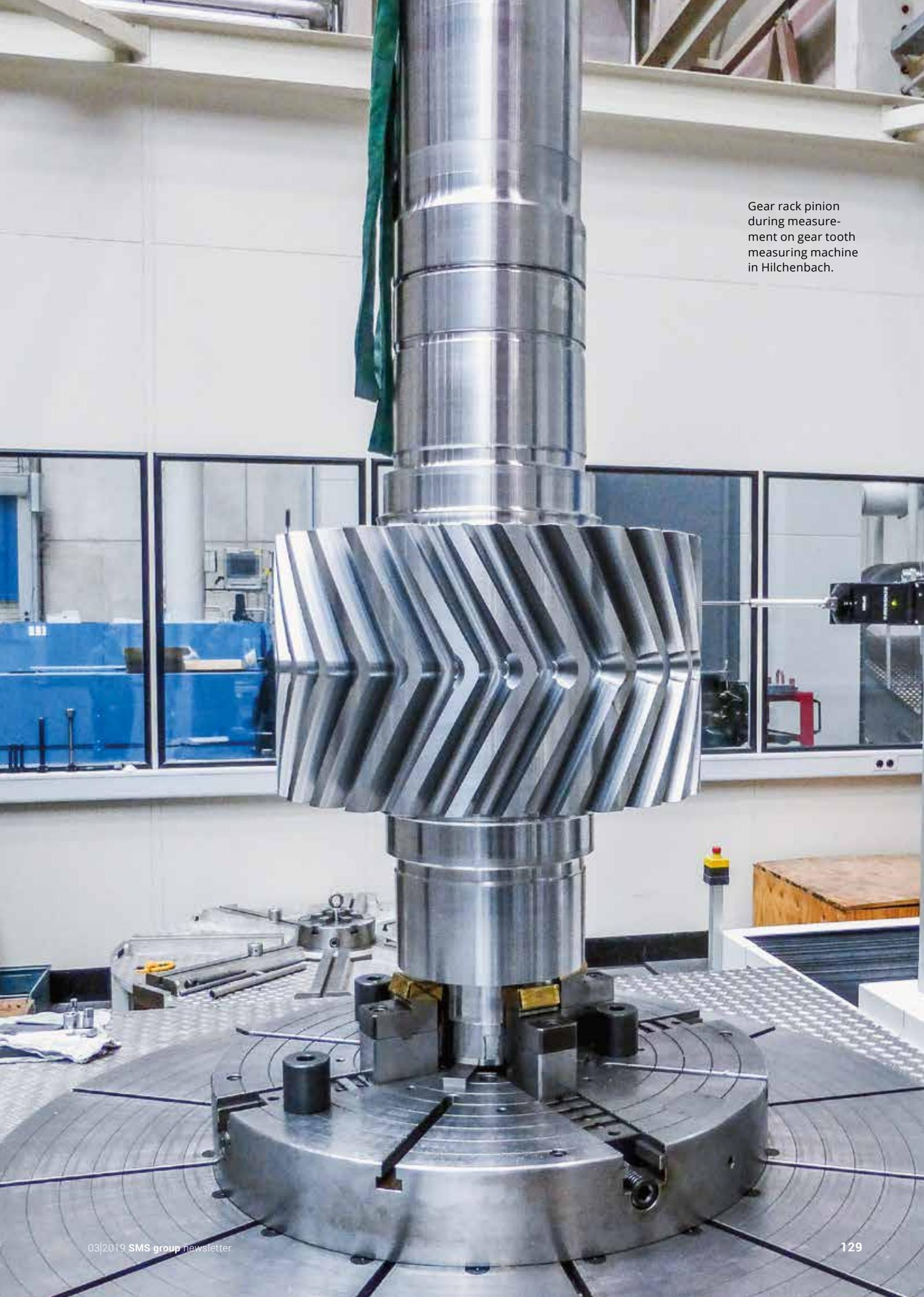
Gear rack pinion during measurement on gear tooth measuring machine in Hilchenbach.
