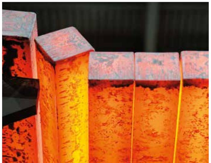
Square blooms cast on a continuous casting machine built by SMS Concast.
