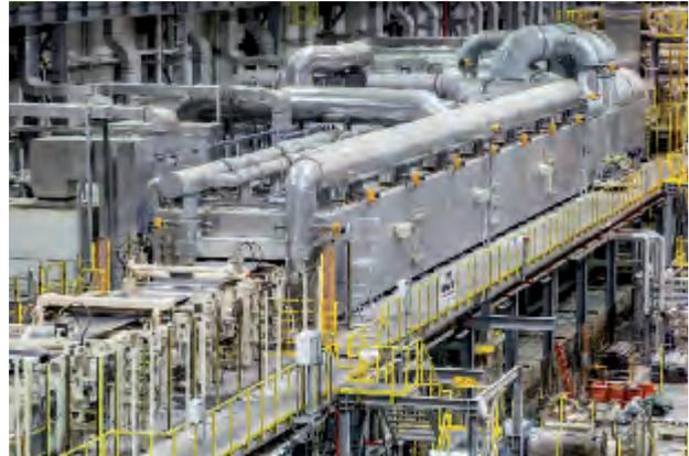
A highlight of the line: the floatation furnace with water quench and floatation air cooler. The strip is transported contact-free, heated to over 550 degrees Celsius and then selectively cooled by air and water. This contactless strip transport makes sure the surfaces are free from scratches.
