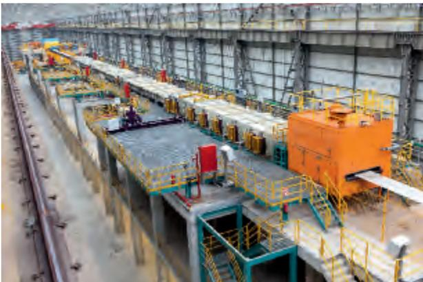
*Completely descaled strip exiting the pickling section.*
