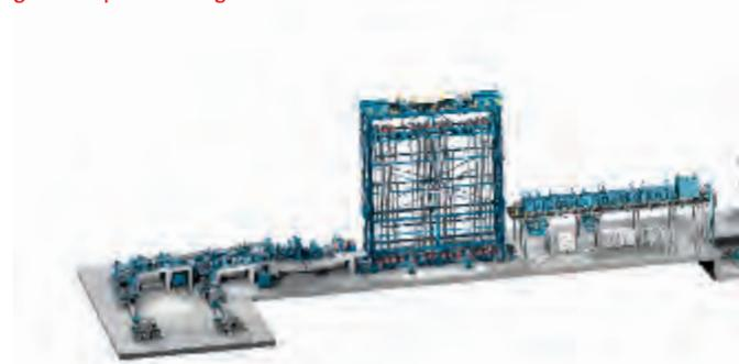
adjustable annealing curves, high cooling rates, and special surface preparation technologies. It meets all the requirements for annealing and subsequently coating a large range of products, including modern high-strength steel grades. Systems for changing the zinc pot as well as state-of-the-art air knives provide the option of different strip coatings.
