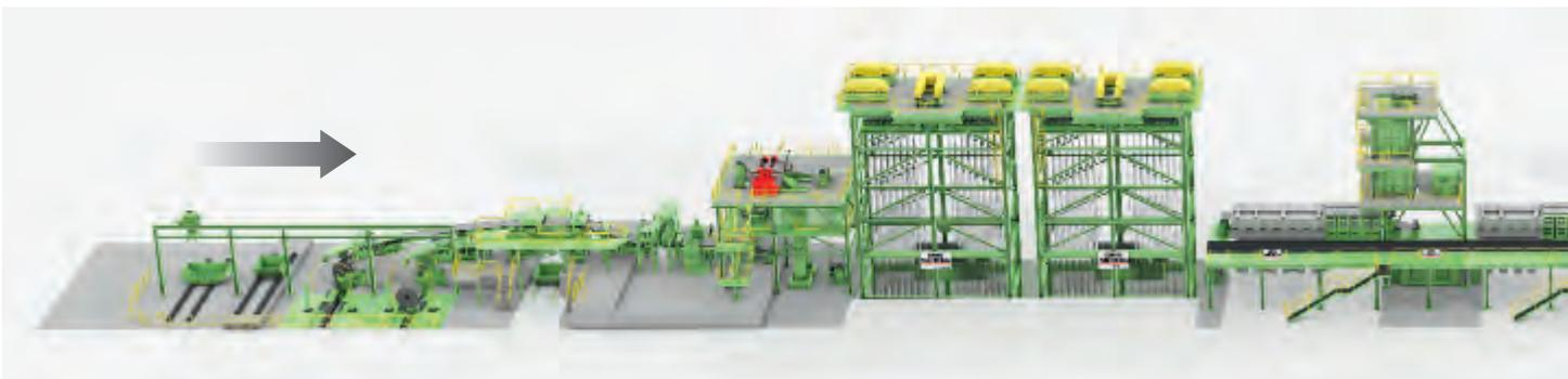
Two 4-high skinpass mill stands are integrated for post-treatment. The first skinpass mill stand adjusts the mechanical-engineering characteristics of the strip by a thickness reduction. The second creates a defined strip surface structure.
