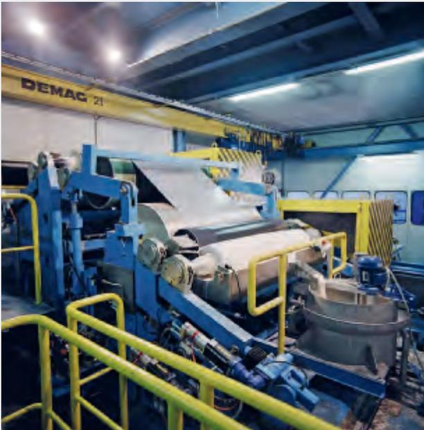
*Roll coaters coat the strip precisely with an insulating layer.*
