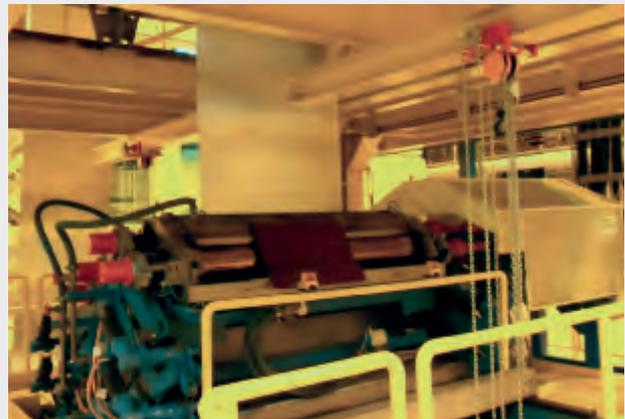
In the vertical coater, the strip is prepared for the next coat with a conversion coating.
