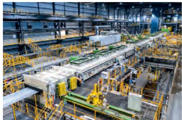
The turbulence technology in the shallow tanks achieves a maximum pickling effect with a minimum of acid and energy.
