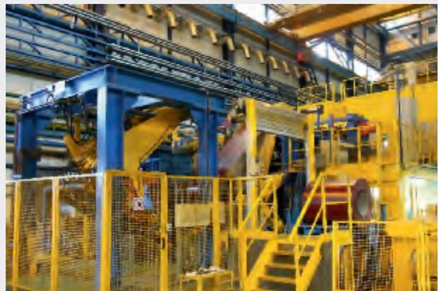
In the exit section, the strips are gently coiled by a belt wrapper and then removed.
