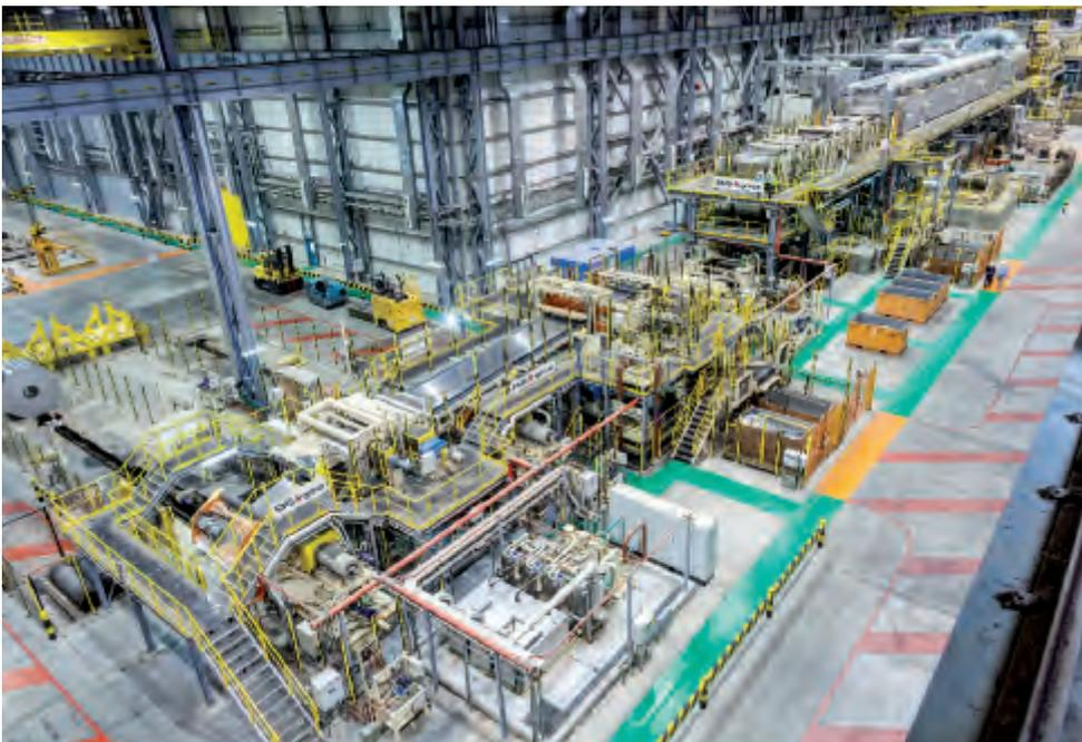
*The new heat treatment and chemical coating line is designed to process cold rolled aluminum strips. The strips are provided with optimum metallurgical properties and surface coatings as demanded for applications in the automotive industry.*
