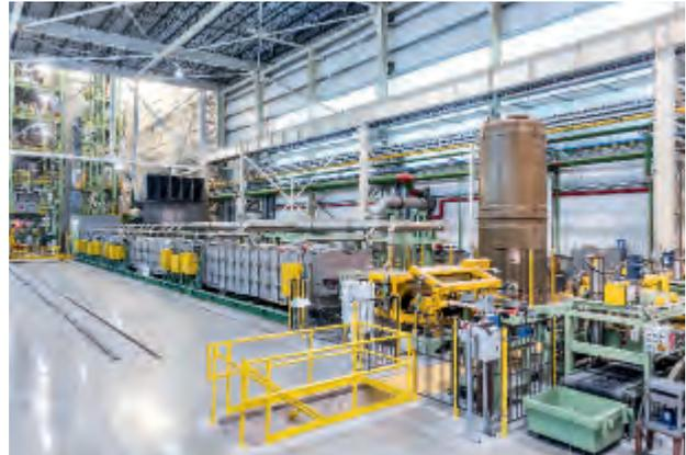
*In a two-stage cleaning section, the cold rolled strip is efficiently freed from rolling oil and other dirt particles.*
