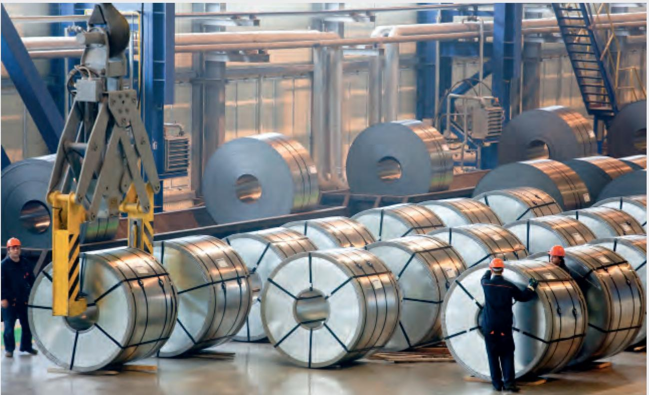
*Pickled and cold-rolled coils for the market or further processing in galvanizing or annealing lines.*
