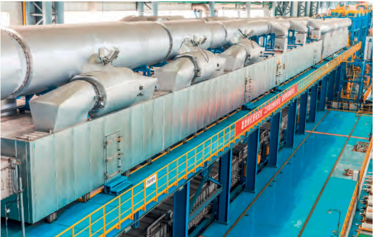
Another highlight of the line is the floatation oven with downstream cooling section. Over a length of more than 100 meters the strip is kept floating, dried and cooled.
