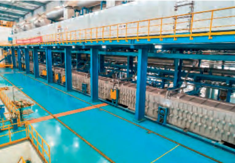
Everything in the line is geared to maximum surface quality. That is why the strip treatment process starts with thorough alkaline pre-cleaning and rinsing. Prior to coating, a second cleaning process takes place in the main cleaning section. There, the layer of oxide is removed by means of alkaline and acid solutions, and the surface is activated for coating. A preparatory chemical is applied in the chemcoater.
