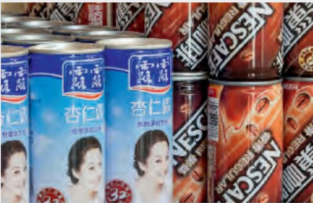
surface-treatment has been carried out. Due to the main application of tinplate being packing material, it is also known as “packaging steel”. Tin cans for foodstuffs, pet food and beverages are a main area of application. Packaging for chemical-engineering products and spray cans for aerosols are also made from this thin material. Furthermore, closures such as lids and crown caps are often made from tinplate.
