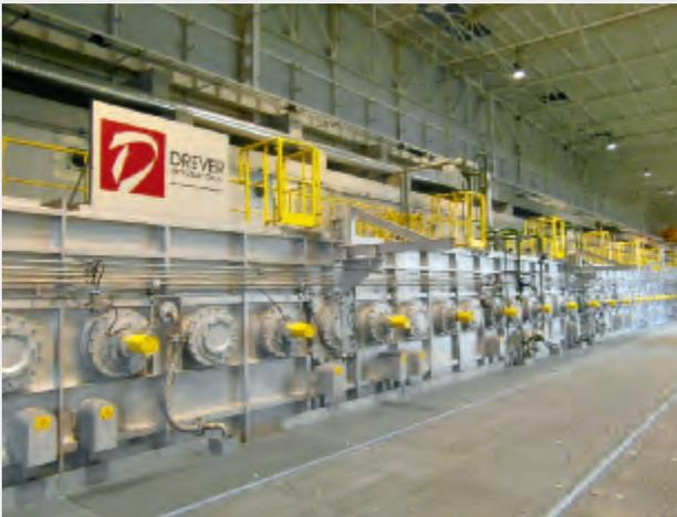
*The horizontal furnace by Drever in the new annealing and coating line for St-Chély d'Apcher.*
