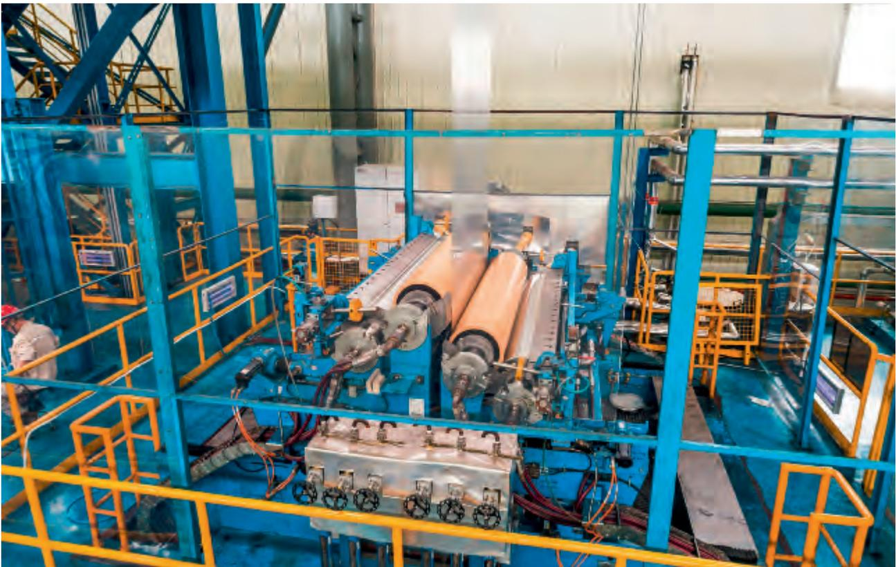
*A heated, vertical roll coater is integrated in the exit section allowing a layer of wax to be applied to the strip as an option.*
