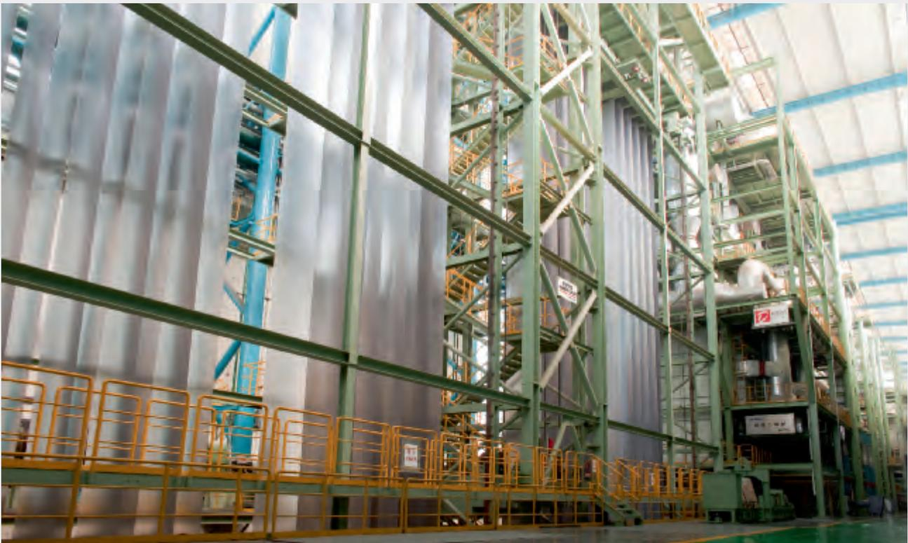
*SMS group's strip processing lines feature large vertical strip accumulators which ensure a high and constant strip speed in the process section in order to achieve high capacities.*
