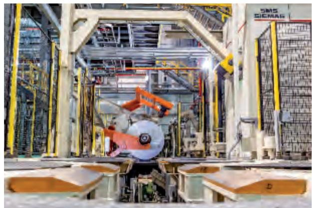
The heat-treated and chemically coated automotive plate arrives at the coiler with belt wrapper. The high-quality aluminum strips are coiled on spools. The complete process is controlled and supervised by the X-Pact® electrical and automation systems from SMS group.
