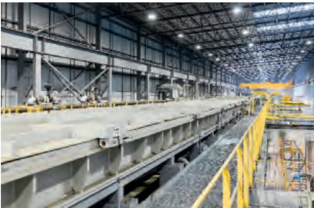
*The turbulence pickling section comprises three plastic tanks and is characterized by high performance at low operating costs.*
