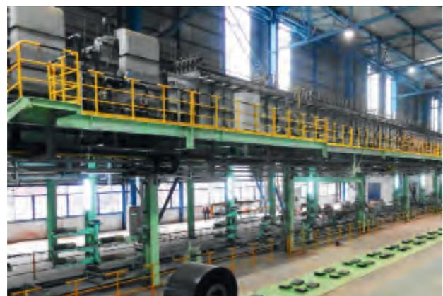
*Furnace for thermal strip flattening.*
