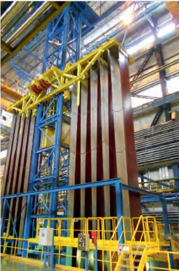
Color-coated strip in the strip accumulator at Severstal.
