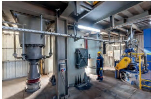
*In the acid regeneration plant, the used pickling acid is recycled and returned to the process.*
