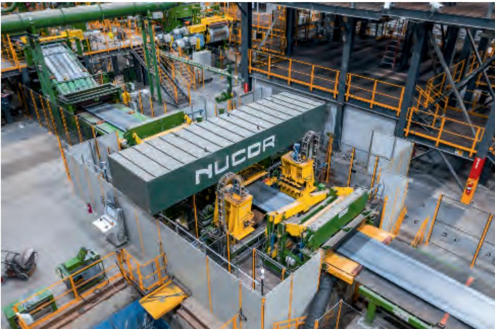
The latest generation of X-Pro® laser welding machine safely and quickly welds together the individual steel strips to produce endless strip. An efficient solid-state laser is used for this purpose.
