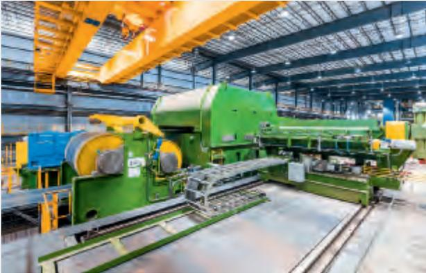
*A scale breaker breaks up and removes some of the scale and increases the flatness upstream of the pickling process.*
