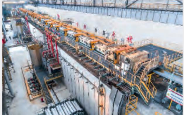
*Pickling sections consist of three to four pickling tanks with own circulation systems.*
