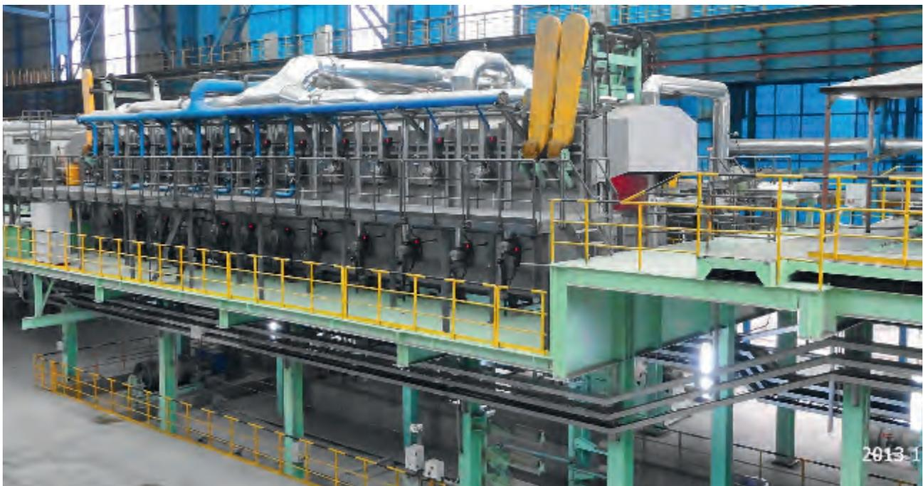
*Catenary furnace for contact-free drying of the insulation layer.*
