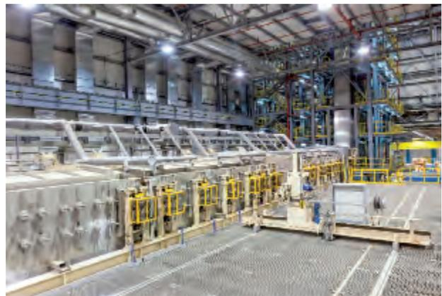
The next step is the cleaning section where rolling oils, other impurities and aluminum oxides are completely removed from the strip surface at minimum media consumption. This section comprises one alkaline and one acid spray cleaning zone each followed by cascade rinsing.
