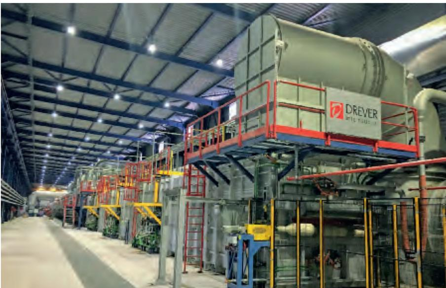
*The powerful furnace from Drever International, member of SMS group, is designed for the resource-saving and efficient processing of cold strip.*
