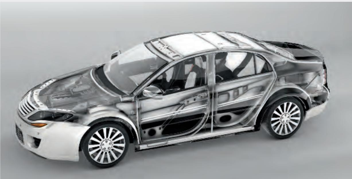
*In automotive construction, a growing number of steels with higher strength and good forming properties are being used.*
