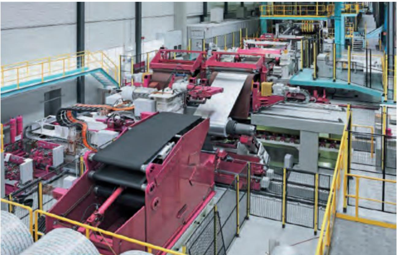
*Exit section of the heat treatment line of AMAG Rolling.*
