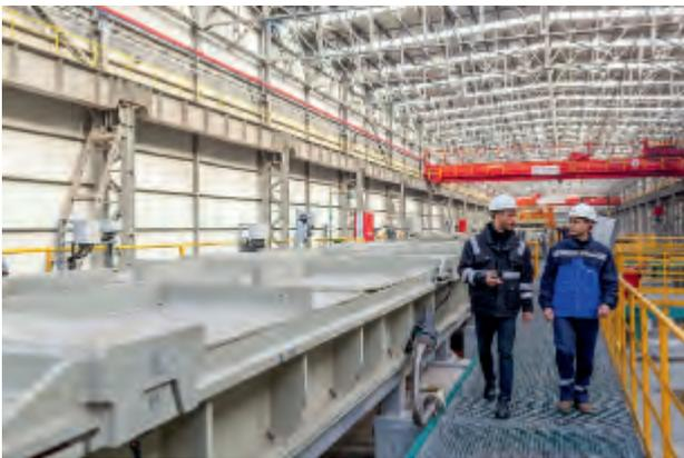
*In the turbulence pickling section, the strip is completely descaled with low resource consumption.*
