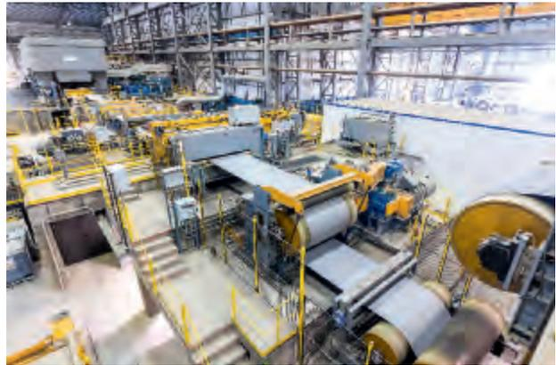
*Combined pickling line/tandem cold mill.*
