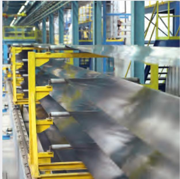
*Horizontal strip looper in an annealing and coating line for NGO silicon steel strip.*
