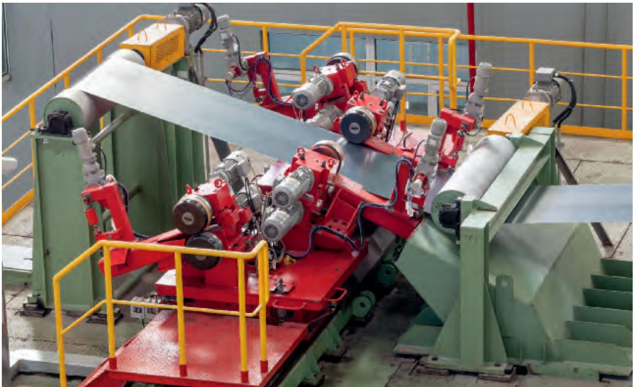
*A special side-trimming shear straightens the strip edges prior to the tinning process.*
