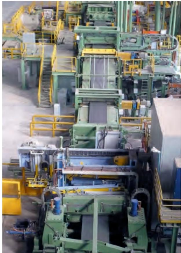
*Upon entering the line, difficult-to-weld steel grades are also joined by an X-Pro® laser welder without the use of filler metals.*
