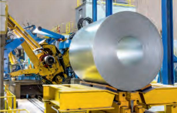
*High-grade, galvanized hot strip on the galvanizing line made by the SMS group at Steel Dynamics Incorporated in Mississippi, USA.*
