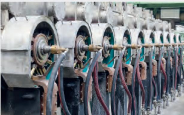
during the transfer of the charge. The thickness of the tin layer can very easily be adjusted via the magnitude of the electric current and via the processing time, which depends directly on the strip speed. Very thin layers of just a few  $\mu\text{m}$  can thus be applied very precisely. Depending on requirements, differing layer thicknesses can also be applied to the strip sides.
