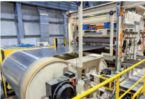
Having a force of 50 tons, the tension leveler can be operated in two modes, without changing the cassettes, depending on the material used: in the stretch bending mode and in the pure stretch mode. The result is an excellent flatness of the strips produced.
