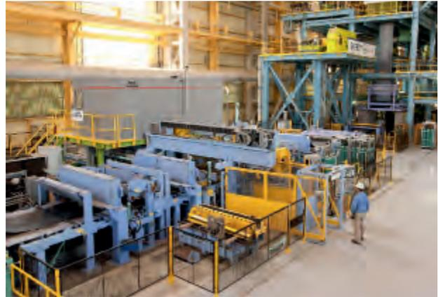
*Upon entry to the continuous pickling line, an X-Pro® laser welder reliably joins the hot-strip ends to form an endless strip.*
