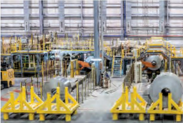
Entry section: two payoff reels ensure the line is continuously fed with strip. The entry side coilers as well as those in the exit section are equipped with manipulators and spool handling system. A downstream stitcher connects the strip heads and tails to an endless strip.
