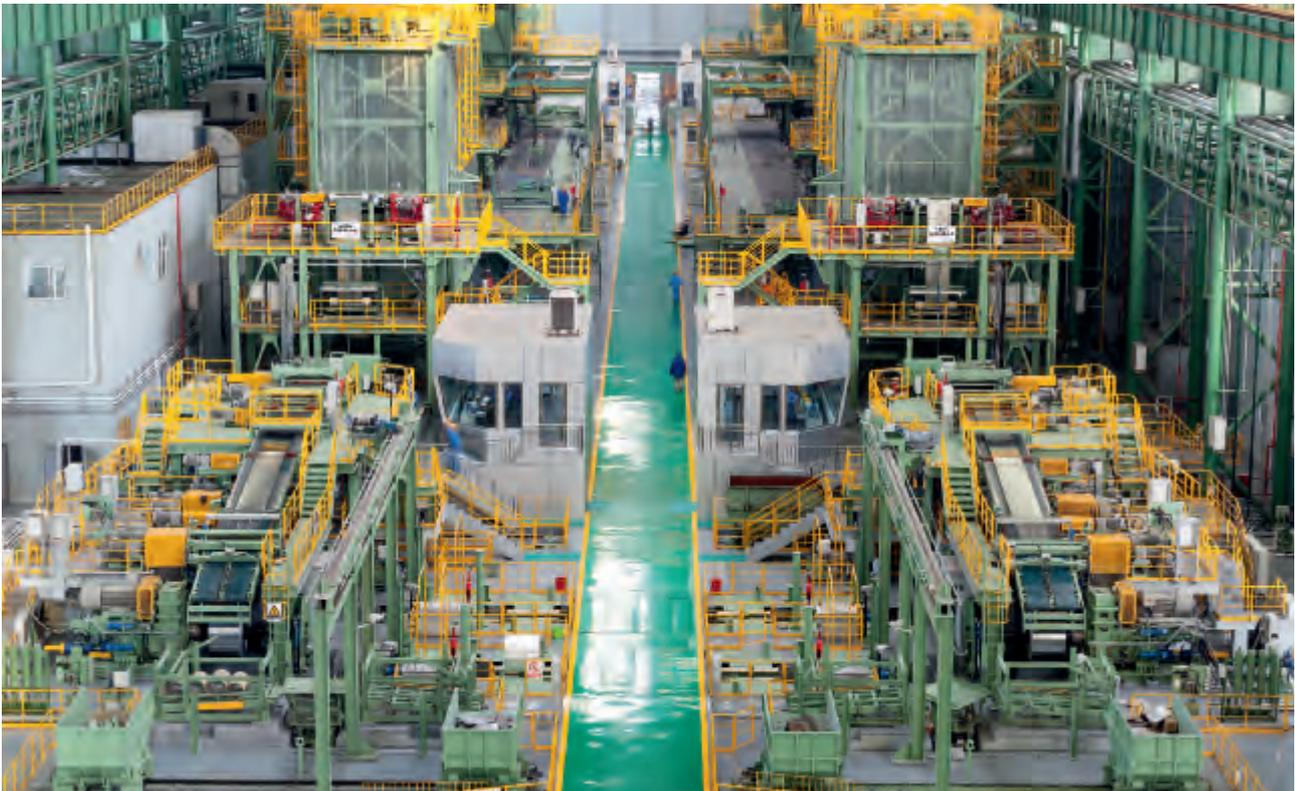
*A total of almost 500,000 tons of high-grade tinplate can be produced by the two tinning lines for the manufacturing of packaging material.*
