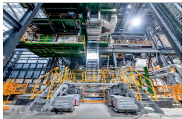
FOEN® air knives continuously ensure a highly precise layer thickness. As soon as the galvanizing is completed, another induction unit can be run into the line. This enables Nucor Gallatin to produce so called galvannealed surfaces, which is a world first in a „heat-to-coat“ line.
