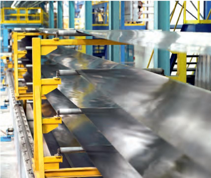
*Horizontal strip looper in an annealing and coating line for non-grain oriented electric steel strip.*
