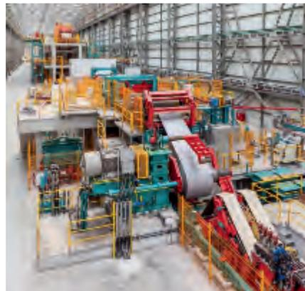
*The strip is safely coiled by a belt wrapper, without clamping.*
