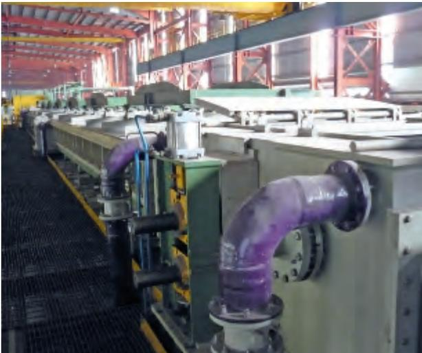
*In a turbulence tank pickling section, more than 100 meters long, the strip is completely descaled using few resources.*
