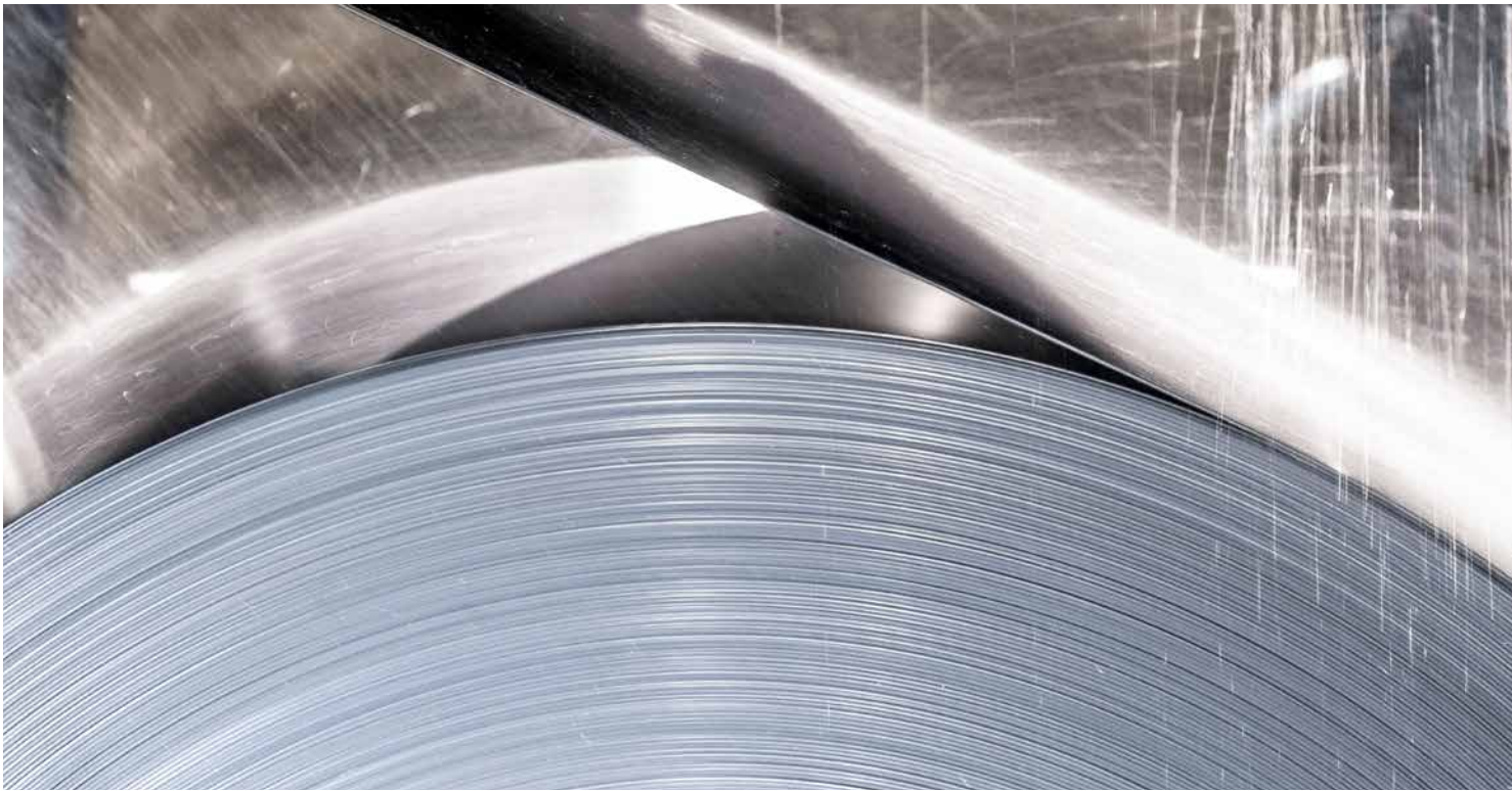
The facility at PTKS produces hot strips between 600 and 1,650 millimeters wide and 1.4 to 16 millimeters thick.
