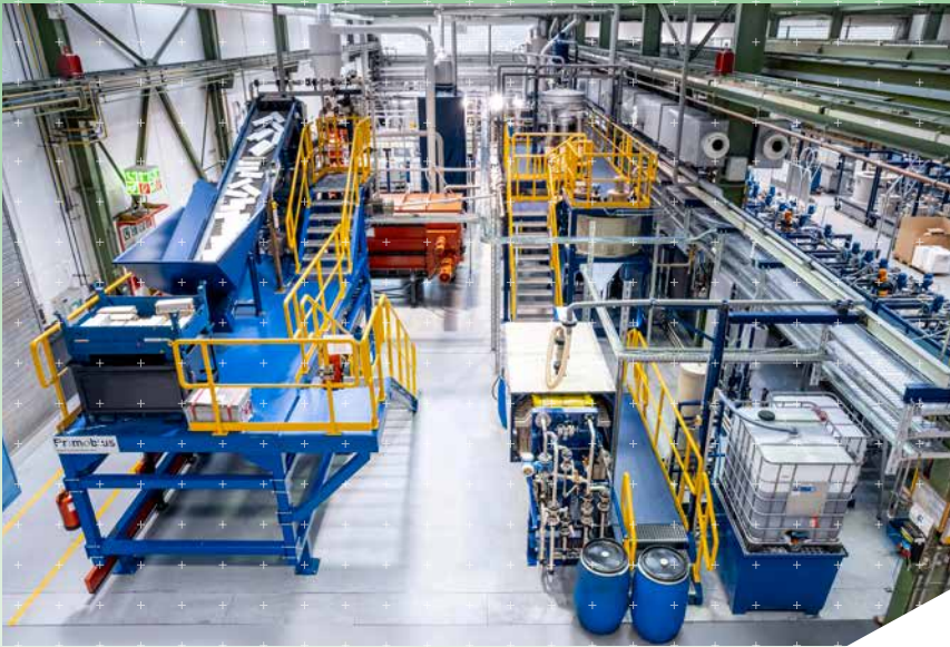
Primobius battery recycling combines mechanical and hydrometallurgical processes.
