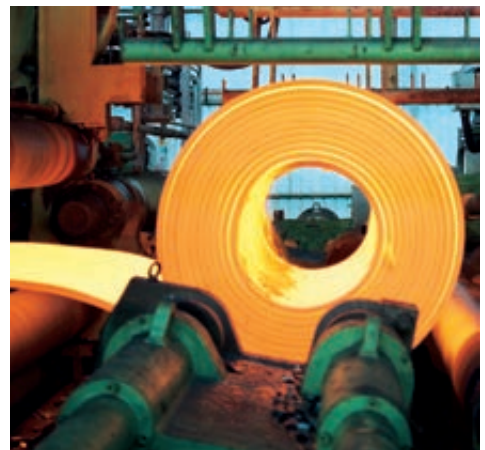
Coilbox uncoiling station.
