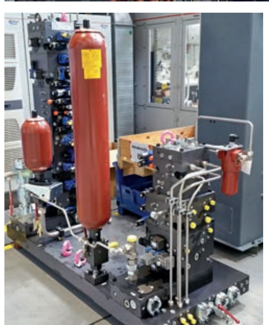
Hydraulics test stand.
