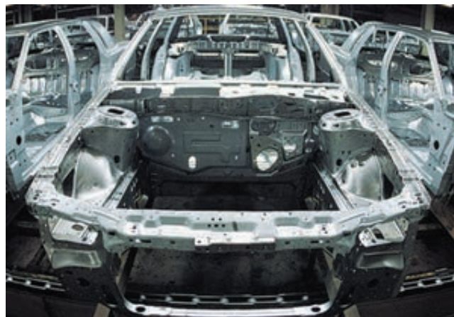
Example of use of AHSS steel grades.
