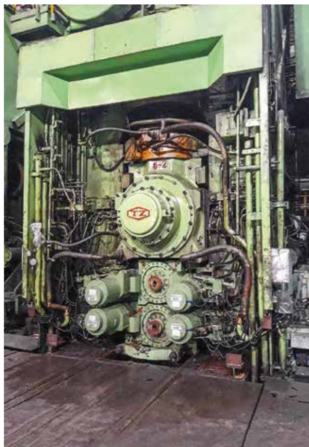
One of the finishing mill stands of Benxi Iron & Steel's hot strip mill after the installation of the CVC®plus system.
