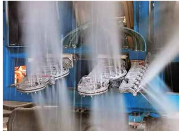
The die lubrication system with additively manufactured spray heads.
