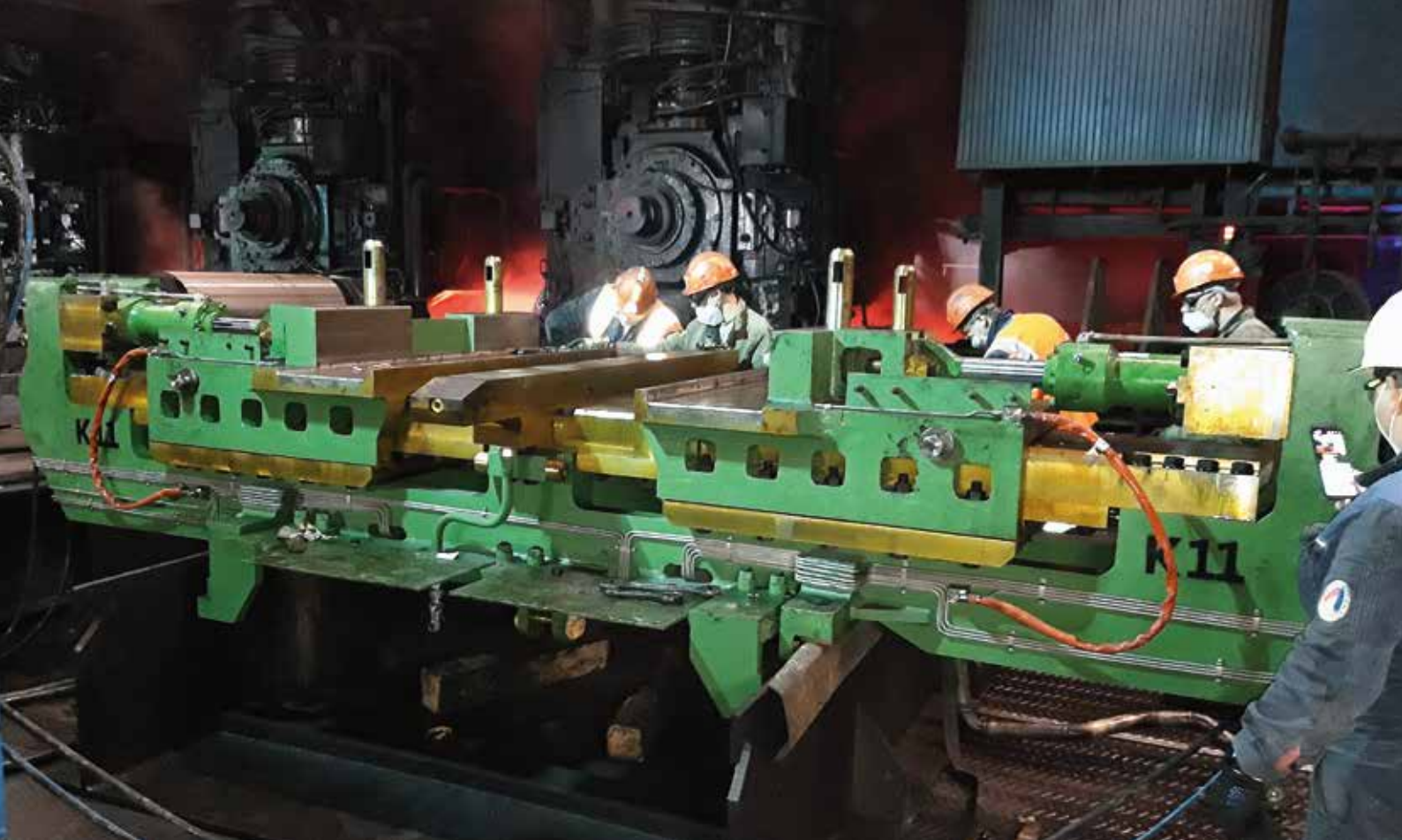
An intermediate-stand base frame dummy was used for pre-assembly and function-testing of the new equipment during ongoing production. The new hydraulic valve stand was also operated in this phase.
