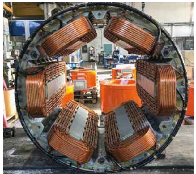
CONSTIR ReNew turns old into new: worn coils (top), and newly installed coils as part of a complete renewal (bottom).
