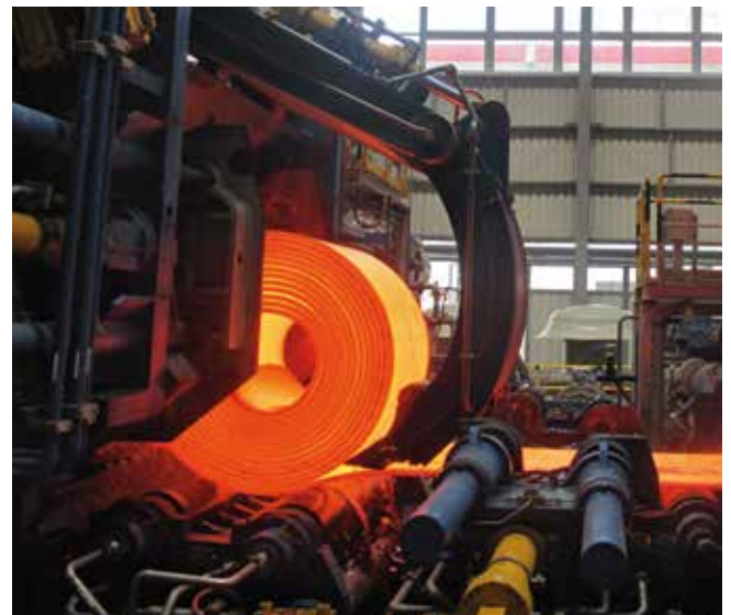
The mandrel-less coilbox reduces temperature losses of the transfer bar, especially at the inner windings.
