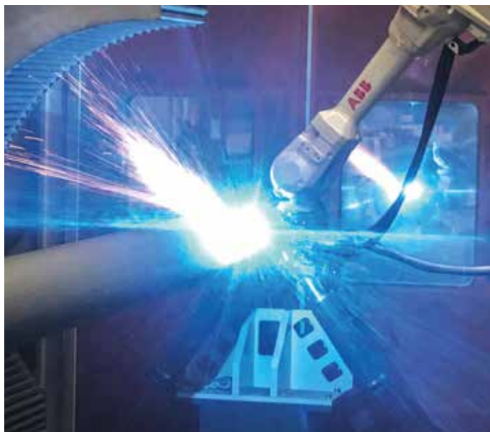
Thermal coating of a mandrel bar by means of PERFECT spray®.
