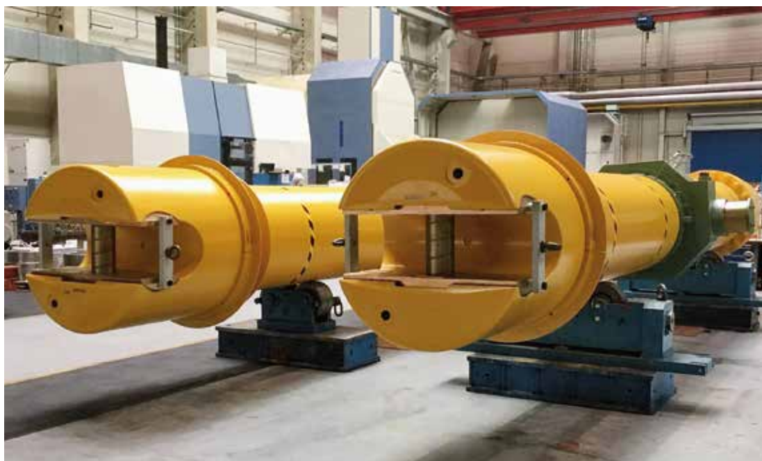
The flat-neck spindles from SMS group ensure the safe and efficient transmission even of extremely high torques. (Photo taken during the workshop assembly.)
