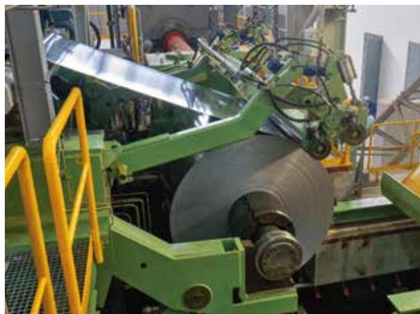
The first strip had a width of 1,780 millimeters and was rolled to a final gauge of 2.8 millimeters.
