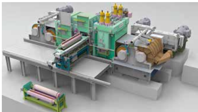
Designed for hot strip with yield points over 1,000 megapascals: scale breaker SB-80-V1050 made by SMS group.
