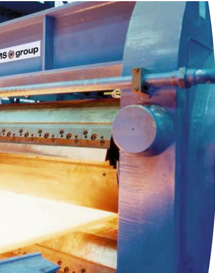
Top: Drum-type shear with hydraulic knife clamping device in a hot strip mill.
