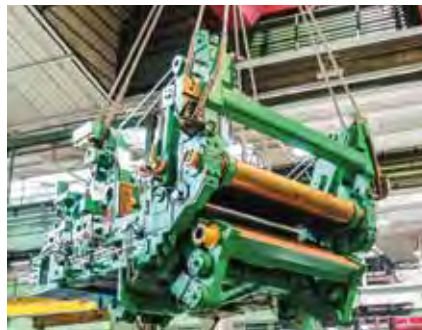
1 Loading of a pinch roll unit with bending devices after workshop assembly.
