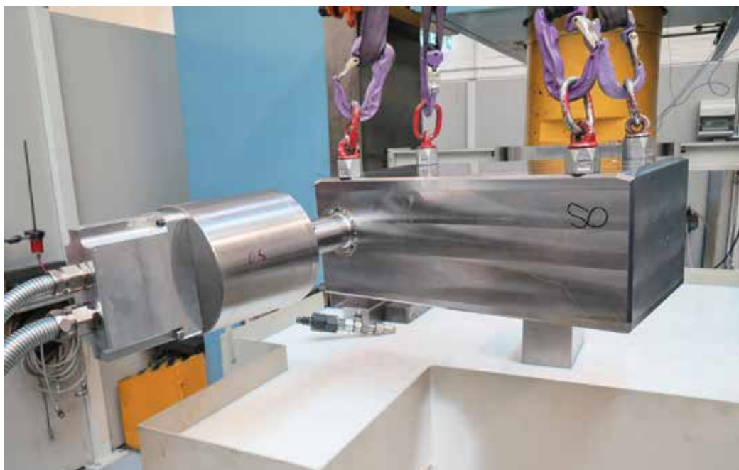
Actuator box during a test in the SMS group Hilchenbach workshop.
