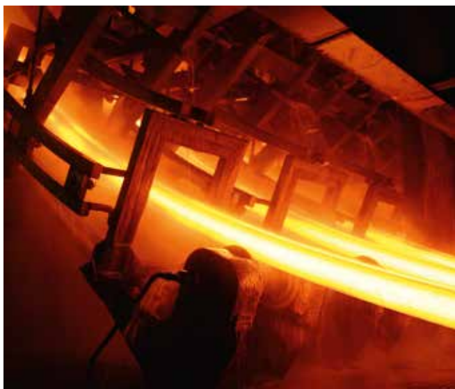
The cooling chamber of a billet caster.
