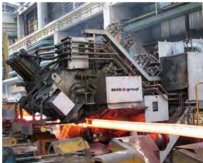
EBROS system during welding process used in production.
