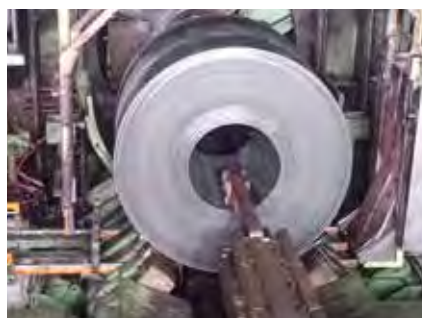
3 Clamping in the coil eye.
