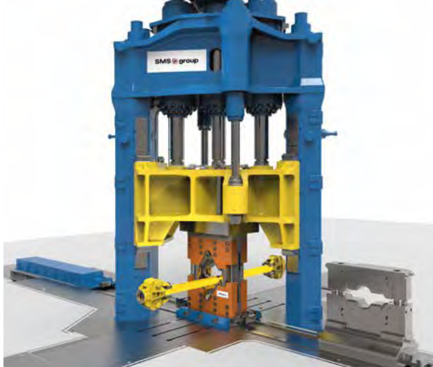
50/55-MN open-die forging press of two-column, push-down design with fitted X-Forging Box.
