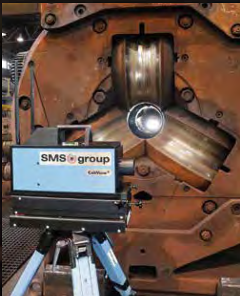
CaliView ® measuring system for inline calibration of the rolling mill and the passes.
