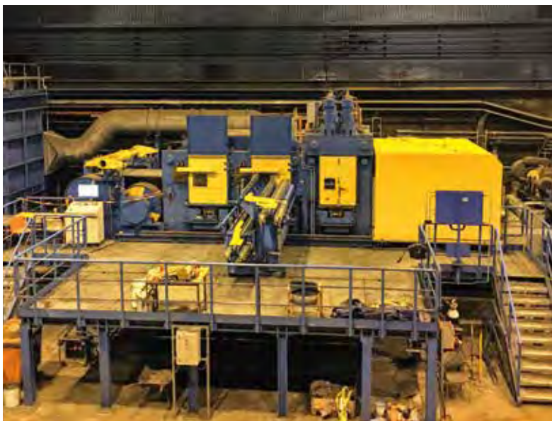
The scale breaker is designed to process high-strength strips.
