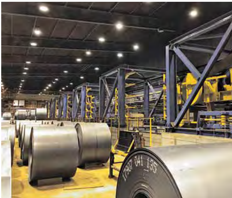
The horizontal six-fold looper is capable of accumulating 410 meters of strip and allows a constant process speed of 180 meters per minute to be maintained while the coils are being welded together in the entry section.
