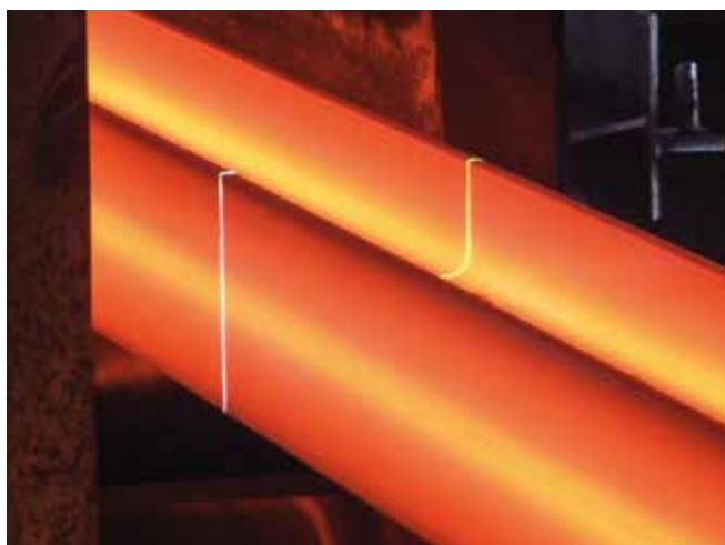
Laser-based dimension measurement and surface inspection on hot H-beam.
