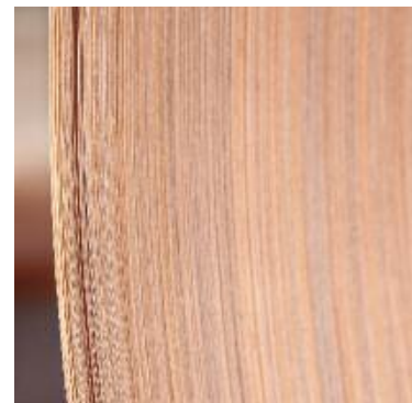
... just as effectively as thin strip. The material is then precisely wound into coils weighing a maximum of 5 t.
