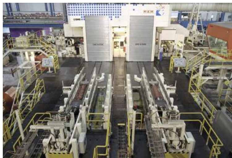
The two-stand tandem mill at MKM rolls a wide range of materials and gauges.
