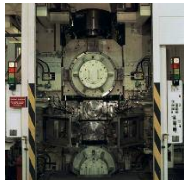
The two four-high roll stands comprise the technological core unit of the line.
