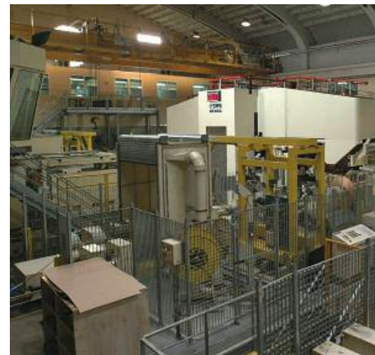
The first copper cold rolling mill from SMS with a system for sle... that ensures high horizontal stabilization of the output. It is ope...
