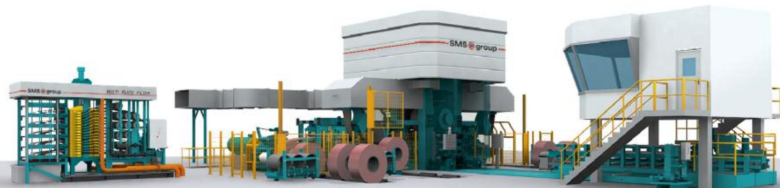
Design of a six-high reversing cold rolling mill with CVC® plus and Multi-Plate® filter for copper strip.
