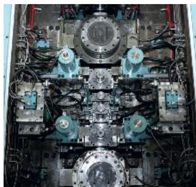
Six-high mill stand with CVC®plus.
