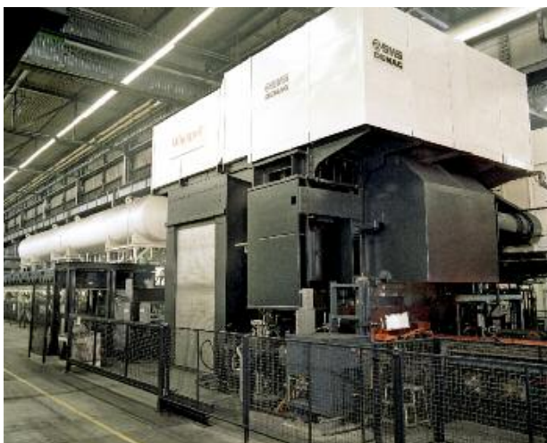
SMS group thoroughly revamped the hot rolling line of Wieland Werke AG in Germany. The core unit is the two-high reversing hot rolling mill.
