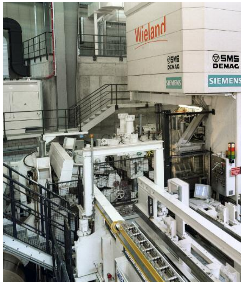
The Wieland tandem mill rolls a large spectrum of strip gauges.
