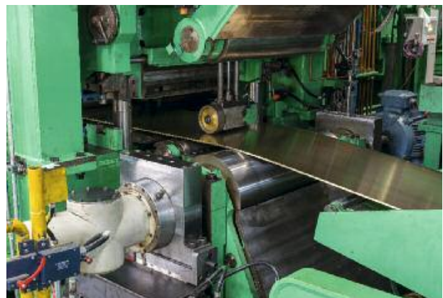
Robust design and precision measurement for excellent strip flatness: the X-Shape flatness measuring roller from SMS group.
