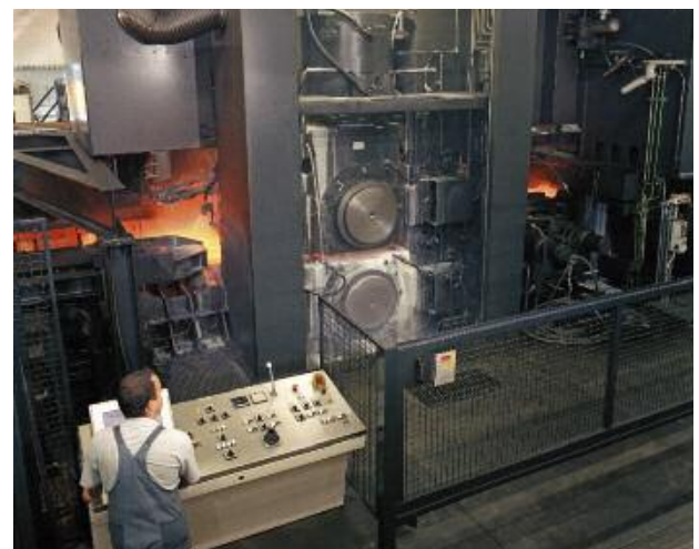
SMS group thoroughly revamped the hot rolling line of Wieland Werke AG in Germany. The core unit is the two-high reversing hot rolling mill.
