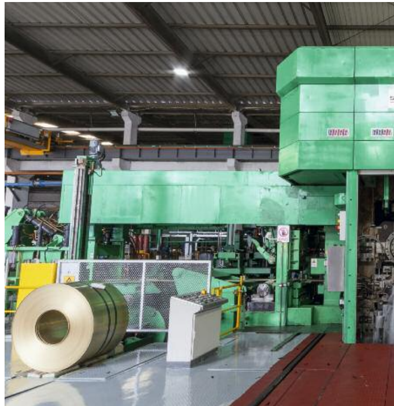
The RCM in four-high design with a combination of payoff gear and payoff drum in the entry and exit sections.
