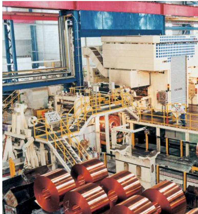
The two-stand tandem mill at MKM rolls a wide range of materials and gauges.
