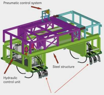
The individual modular units are interconnected via hoses, which means less adaptation work
