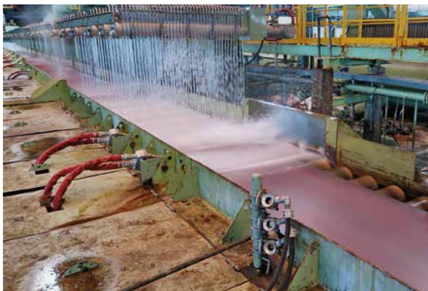
Cooling section at the exit side of Ningbo Iron & Steel's hot strip mill, as modernized by SMS group. The cross-spraying systems were also reinforced in addition to the laminar cooling.
