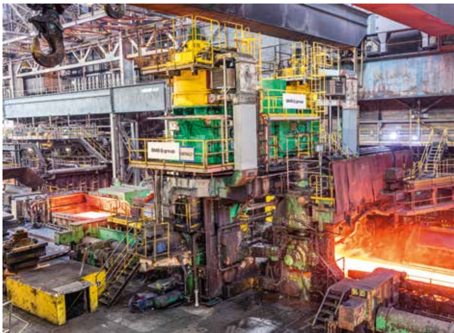
After: Roughing stand with edger after revamp. Exit side view.
