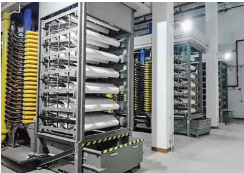
Three Multi-Plate® filters from SMS group clean the rolling oil efficiently and environmentally friendly.
