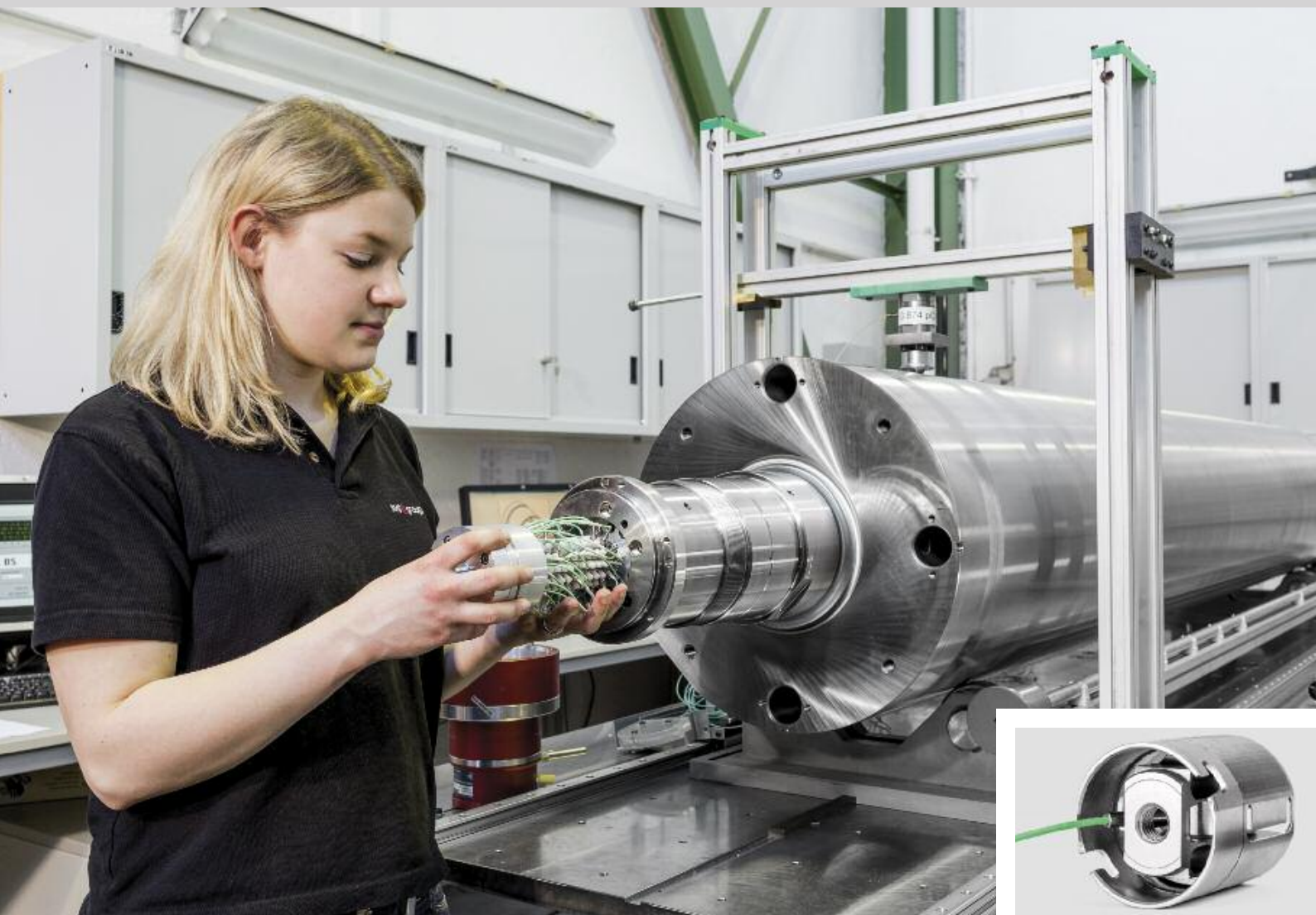
Precise X-Shape flatness measuring system with measuring rollers of the latest generation.
