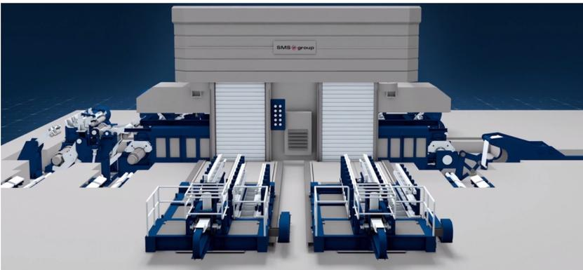
Design concept of a CCM<sup>®</sup> (Compact Cold Mill) by SMS group.
