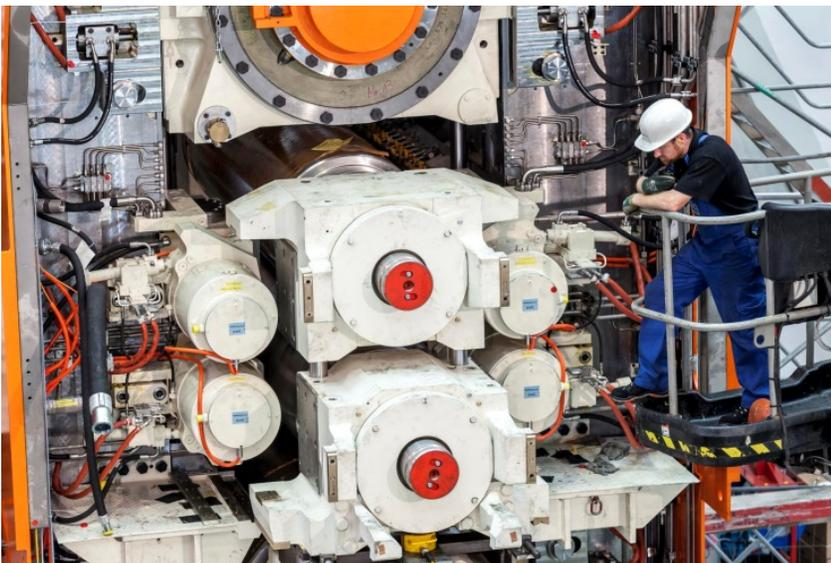
Pre-assembly of a CVC<sup>®</sup>plus system in the SMS group workshop.
