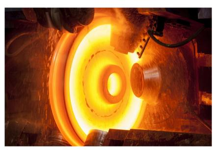
Wheel rolling machine of the type DRAW 1250 forms railroad wheels with 13 CNC-controlled axes to a diameter of up to 1,200 millimeters fully automatically.
