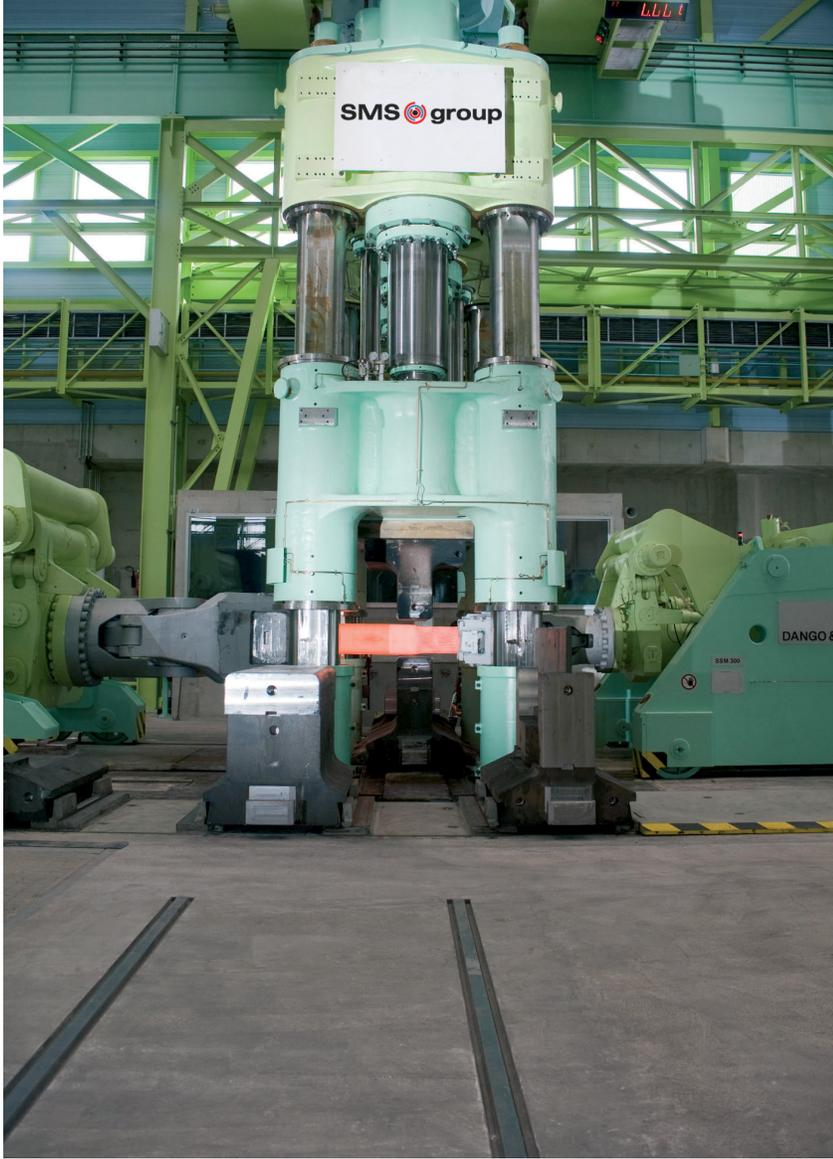
An identically designed open-die forging press from SMS group in operation.
