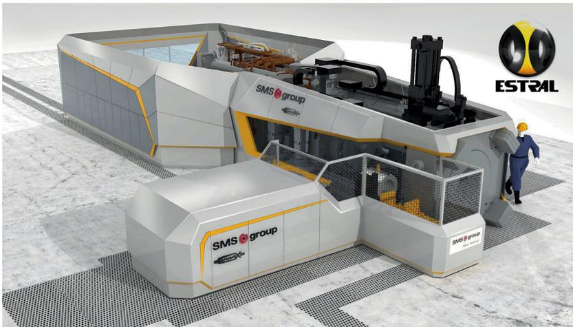
HybrEx<sup>®</sup> extrusion press with new soundproof enclosure.
