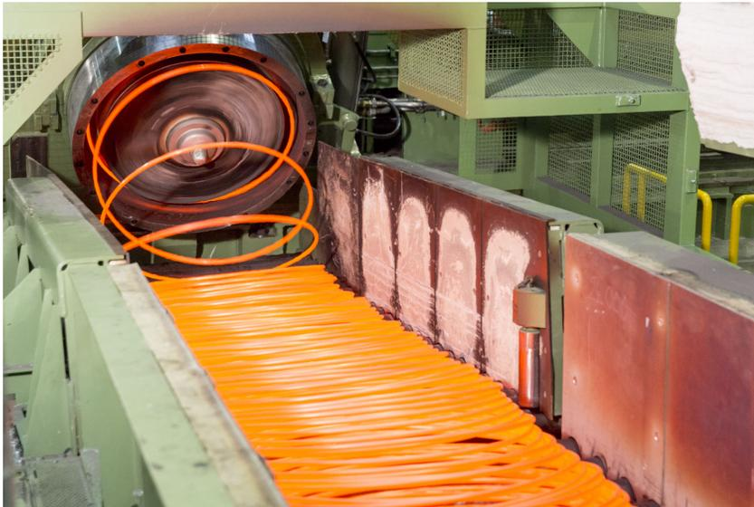
Among others, SMS group will supply to Jianlong Beiman a loop layer for its high-speed wire rod mill.
