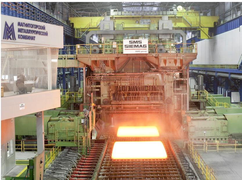
In future, the mill stand will be able to roll slabs up to 350 millimeters thick.
