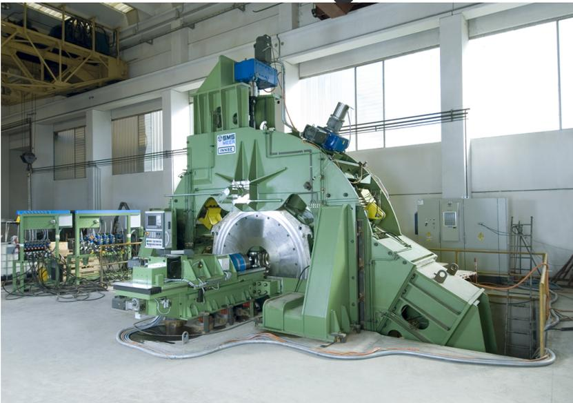
3-in-1: The new PQF<sup>®</sup> roll redressing machine combines three plant components into one and thus saves space.
