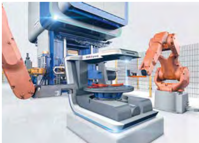
Marking station: a robust data matrix code is applied onto every forged part by dot peen marking.
