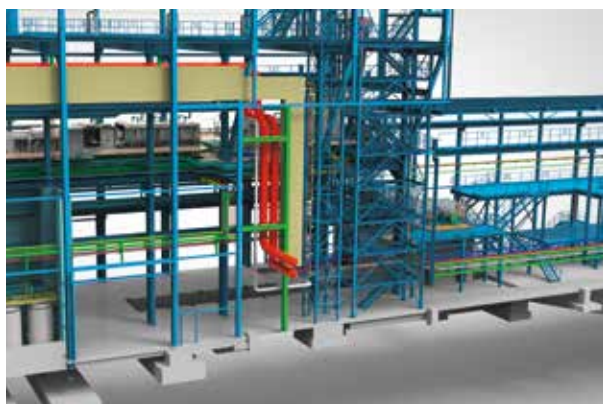
Collision control – shown here are the supporting steel structure, process piping, cable routes and planned walking paths.
