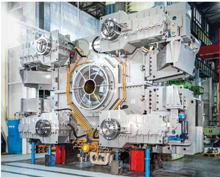
Two tilt drives were replaced at Třinecké Železářny.
