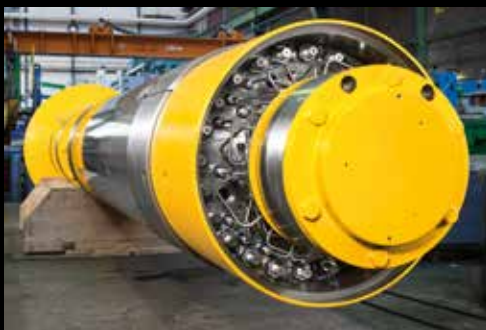
View on optimized grease lubrication system without mounted protective cover.
