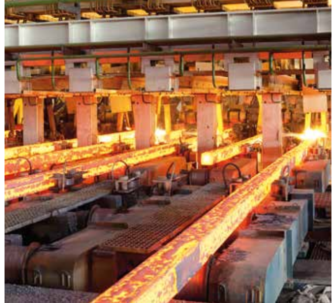
High-speed casting in eight strands on an SMS Concast casting machine.
