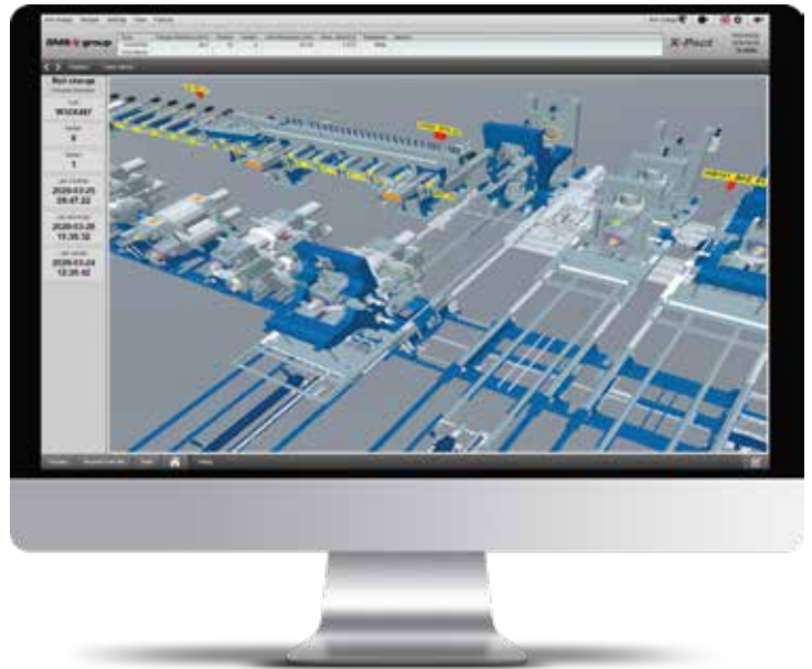
The Digital Twin of the CCS® tandem reversing group for H- and I-beam rolling is a functional and technological replica generated in order to perform real-time near-reality 3D plant simulation.
