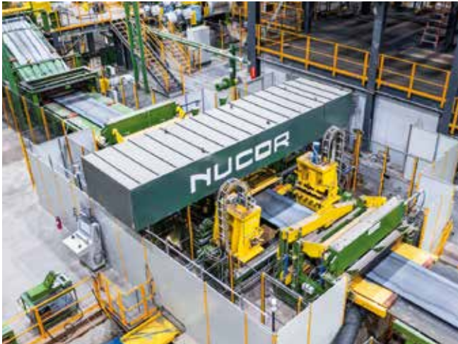
The latest generation of X-Pro® laser welding machine safely and quickly welds together the individual steel strips to produce endless strip. An efficient solid-state laser is used for this purpose.
